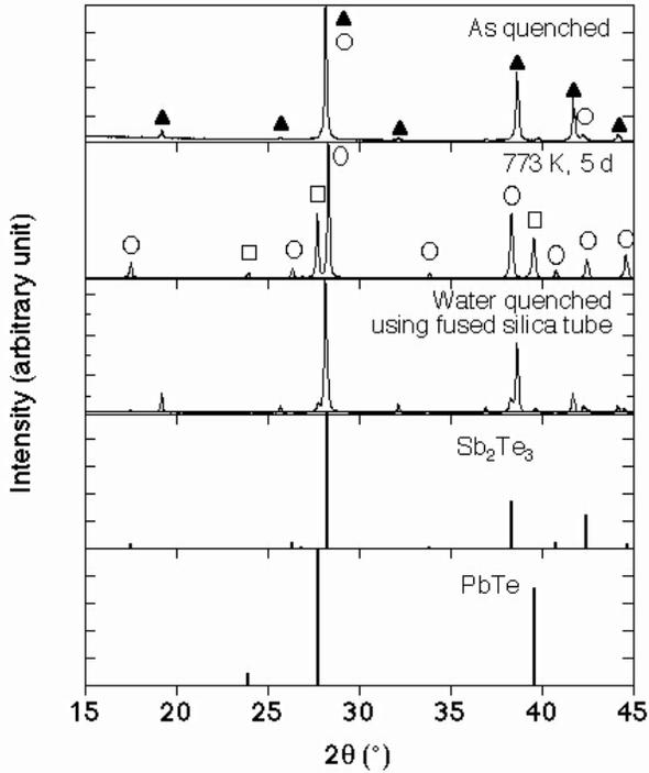
**Figure 2:** XRD profiles obtained from  $\text{Pb}_{10.5}\text{Sb}_{31.6}\text{Te}_{57.9}$  as quenched and annealed at 773 K for 5 days. Open squares ( $\square$ ), open circles ( $\circ$ ) and solid triangles ( $\blacktriangle$ ) show the peaks from PbTe,  $\text{Sb}_2\text{Te}_3$  and  $\text{Pb}_2\text{Sb}_6\text{Te}_{11}$  phases, respectively.
