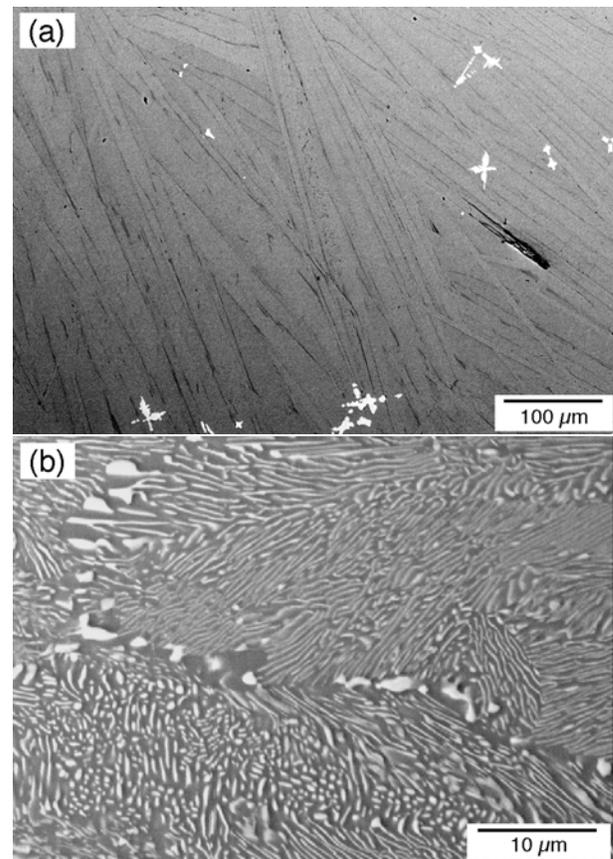
**Figure 1:** Microstructure of Pb<sub>10.5</sub>Sb<sub>31.6</sub>Te<sub>57.9</sub>: (a) as quenched and (b) annealed at 673 K for 150 h.
