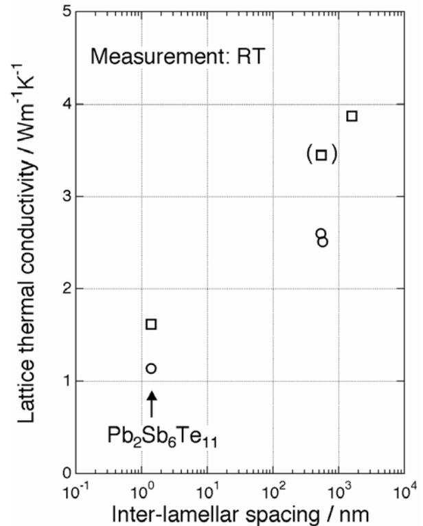
**Figure 5:** The dependence of lattice thermal conductivity of  $\text{PbTe}/\text{Sb}_2\text{Te}_3$  lamellar composites and  $\text{Pb}_2\text{Sb}_6\text{Te}_{11}$  on inter-lamellar spacing. Circles and Squares show the results from samples sample A and B, respectively. The spacing for  $\text{Pb}_2\text{Sb}_6\text{Te}_{11}$  was taken to be the period of similar atomic stacking (1.4 nm) in the crystal structure [She04].
