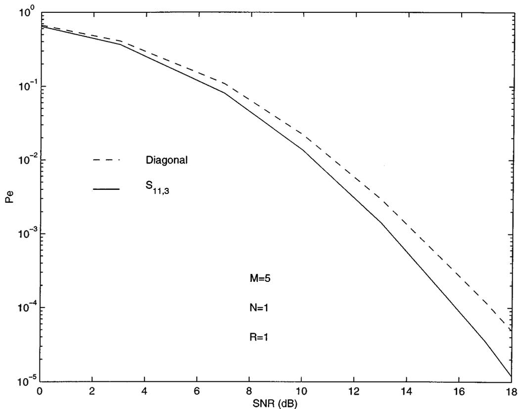
Fig. 8. Block-error rate performance for  $M = 5$  transmitter antennas,  $N = 1$  receiver antenna, and rate  $R = 1$ . The solid line is the nongroup  $\mathcal{S}_{11,3}$  having 33 elements ( $R \approx 1.01$ ). The dashed line is the best  $R = 1$  group construction: in this case the best 32-element diagonal constellation.
