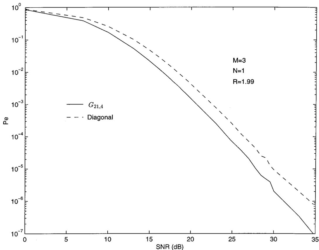
Fig. 5. Block error rate performance of the group  $G_{21,4}$ , which has an irreducible representation of  $L = 63$  matrices for  $M = 3$  antennas ( $R \approx 1.99$ ), and best diagonal (Abelian group) constellation with the same rate, described in Table I, for  $N = 1$  receiver antenna.
