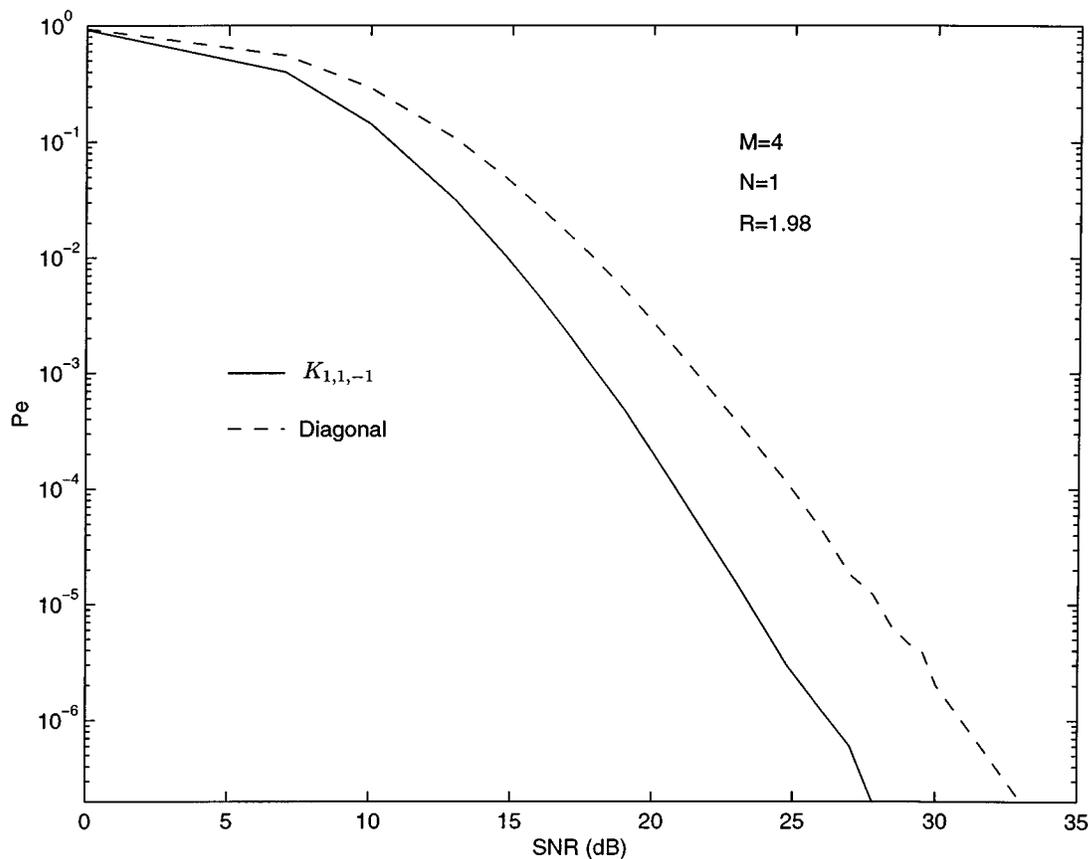
Fig. 7. Block-error rate performance of the group  $K_{1,1,-1}$  compared with the best diagonal code for  $M = 4$  transmitter antennas and  $N = 1$  receiver antenna. The solid line is  $K_{1,1,-1}$  the binary extension of the group  $SL_2(\mathbb{F}_5)$  having  $L = 240$  unitary matrices ( $R \approx 1.98$ ). The dashed line is the diagonal construction with the same rate, described in Table I.
