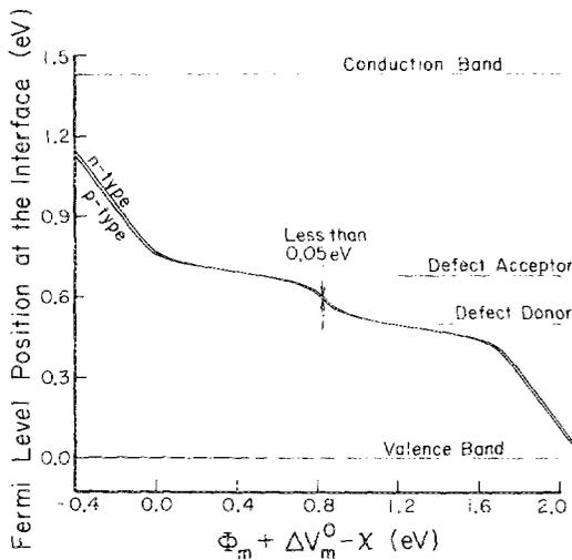
FIG. 2. Position of the Fermi level at the interface vs metal work function ( $\Phi_m$ ) for the case of bulk metallic coverage on *n*- and *p*-type semiconductors.  $\chi$  is the electron affinity of the semiconductor, and  $\Delta V_0$  is the potential difference between the metal surface and bulk.
