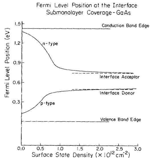
FIG. 3. The position of the Fermi level at the interface vs density of surface donors (and acceptors) for the case of submonolayer coverage on *n*- and *p*-type semiconductors. We assume arbitrarily that there are an equal number of donor and acceptor states.
