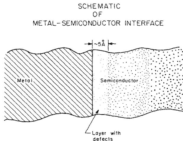
FIG. 1. Geometry of the metal semiconductor interface, including charged interface states.
