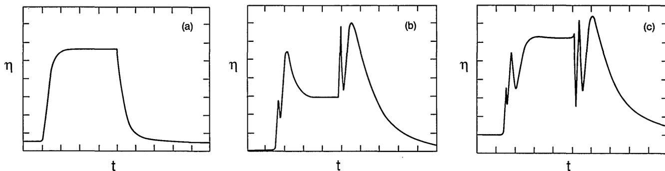
Fig. 3. Diffraction efficiencies recorded during writing and erasure of gratings. The peak diffraction efficiency in each case is approximately  $25 \pm 3\%$  (diffraction efficiency is defined as the ratio of the input readout power to the diffracted power); the horizontal scale is 793.5 msec/division. (a)  $P_1 = 24$  mW,  $P_2 = 2.1$  mW; (b)  $P_1 = 27.8$  mW,  $P_2 = 10.8$  mW; (c)  $P_1 = 20.7$  mW,  $P_2 = 20.8$  mW.
