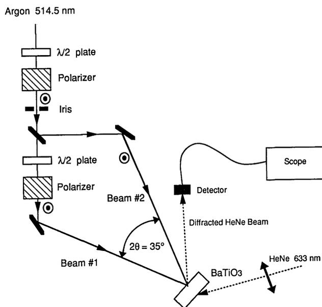
Fig. 2. Apparatus for writing and probing deep holograms.
