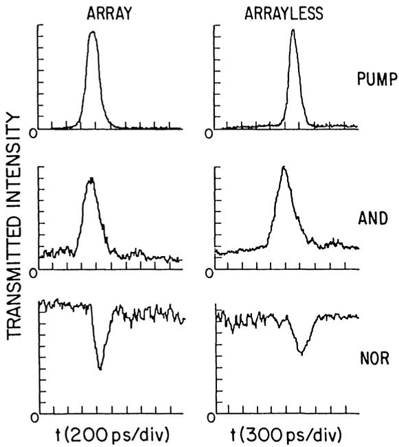
Fig. 2. Streak camera traces of the temporal evolution of the input pump pulse and the cw probe transmission for AND-gate and NOR-gate operation using one  $9\text{-}\mu\text{m} \times 9\text{-}\mu\text{m}$  pixel of the windowless GaAs etalon. The base lines are taken with the probe beam blocked.
