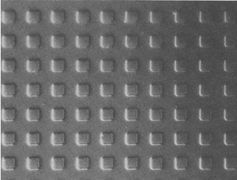
Fig. 1. Photomicrograph of 2-D array of  $9\text{-}\mu\text{m} \times 9\text{-}\mu\text{m}$  pixels prepared by reactive-ion etching.
