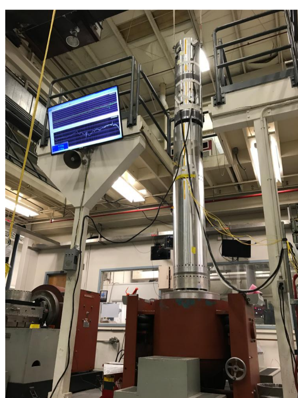
Fig. 5 Payload vibration test at the required vibration level.
