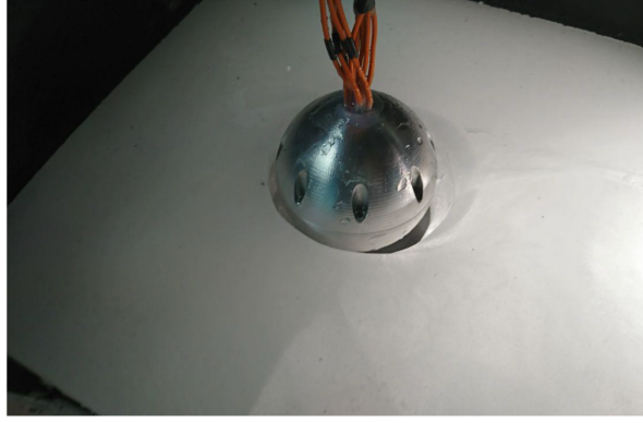
Fig. 2: Snapshot of the experiment as the heated probe starts to melt the ice.
