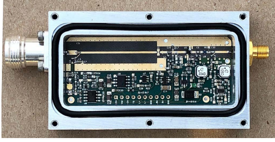
Fig. 1. Amplifier is housed in a water-tight aluminum block with exterior dimensions of 86 \times 54 \times 22 mm 3 .
