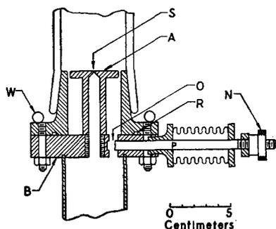
FIG. 1. The anode arrangement of a glow discharge tube showing provision for the control of the pumping speed. *W* is a water cooling line; *R*, a rubber gasket; and *S*, a circular slit 0.1 mm in diameter. The anode *A* screws into *B*. All metal parts are of brass.
