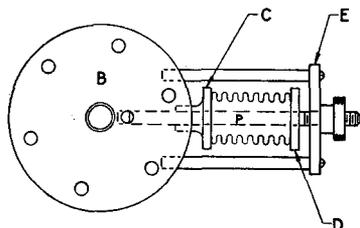
FIG. 2. Plan showing details of the syphon assembly. *P* is soldered to *D* but slides freely through *B*, *C*, and *E*.
