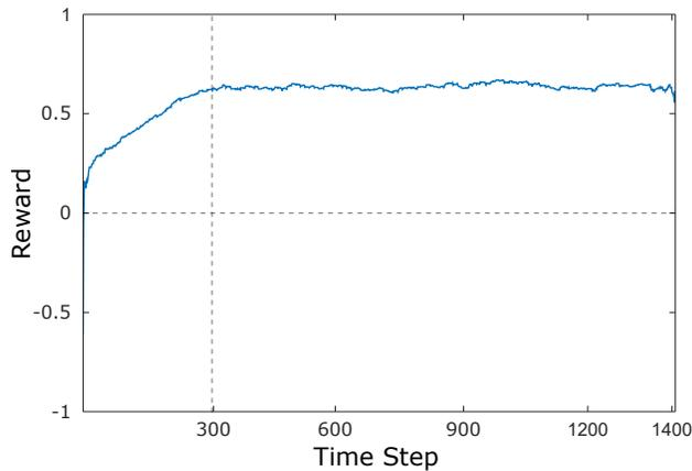
Fig. 5. **The averaged reward increases initially and saturates around 300 time steps.** (Average over 50 simulations.)
