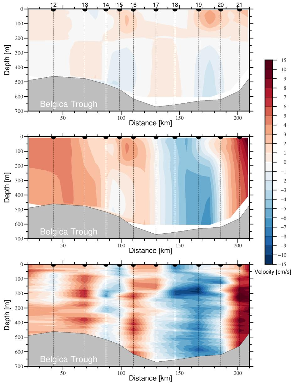
**Figure S2.** Velocities across Belgica Trough shelf-break section, stations 11 to 22. (a) Geostrophic velocity referenced to 300 m, roughly the top of the CDW layer. (b) Geostrophic velocity referenced to the LADCP data as described in section 2.2 of the manuscript. (c) Unreferenced velocities from LADCP data.
