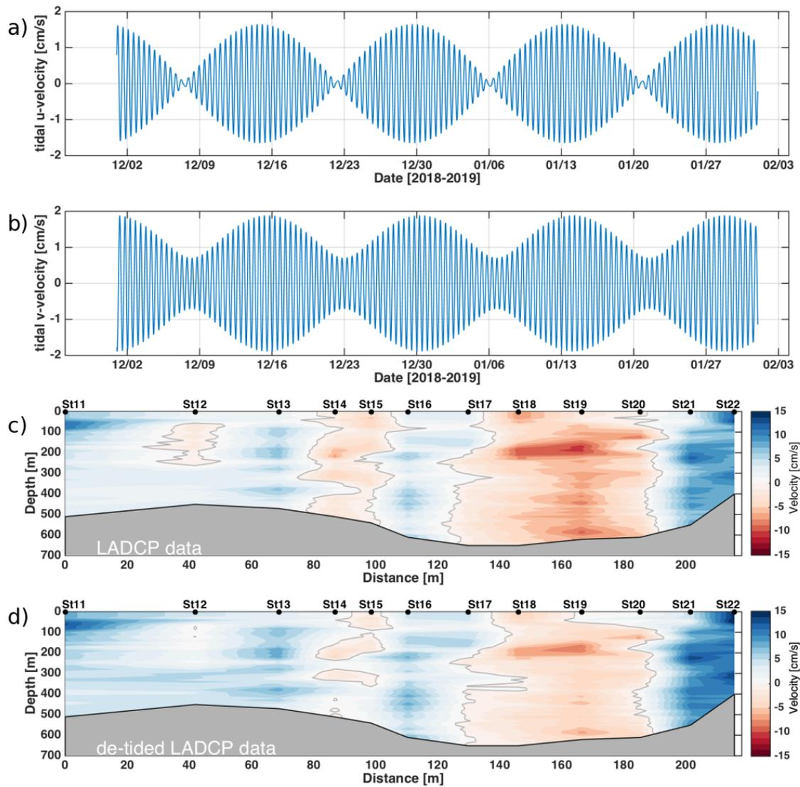
**Figure S1.** Tidal contributions to the LADCP data. (a) Zonal and (b) meridional velocity of tidal flow at station 11 from CATS2008 (Padman et al., 2002), see discussion in section 2.2 Velocity corrections and transports. (c) LADCP velocities and (d) de-tided LADCP velocities across Belgica Trough (stations 11 – 22).
