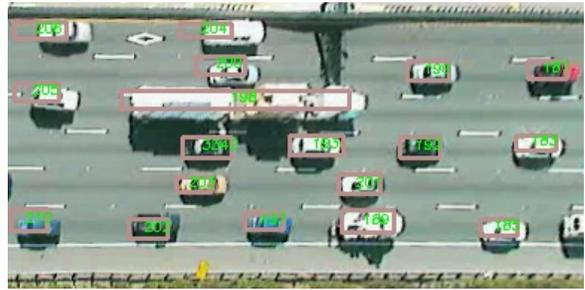
Fig. 5: Sample image of video data from NGSIM showing vehicle positions along with vehicle identification numbers and extracted vehicle dimensions.
