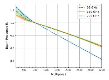
FIG. 6. One-dimensional multipole-space representation of the measured instrument beam,  $B_{\ell}$ , with uncertainties indicated by the shaded regions. The data are normalized to unity at  $\ell = 800$ .
