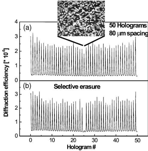
Fig. 2. (a) 50 images recorded in a  $\text{LiNbO}_3\text{:Fe, Mn}$  crystal. Each peak corresponds to the diffraction efficiency of a hologram stored at a different spatial location. (b) Hologram 25 is selectively erased by continuous illumination with UV and red reference light.
