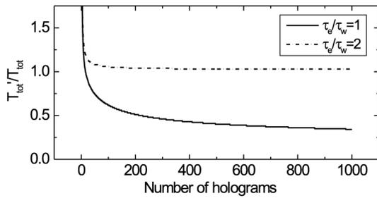
Fig. 3. Ratio of total recording time between the localized and the distributed-volume methods as a function of the number of holograms needed to record for two different values of the ratio  $\tau_e/\tau_w$  and  $t_1 = \tau_e/20$ .
