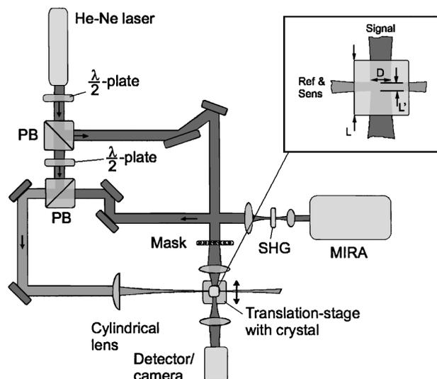
Fig. 1. Recording setup for the 50-hologram experiment. The camera CCD and detector are interchangeable.  $\lambda/2$ -plate, half-wave plate; PB's, polarizing beam splitters; SHG, second-harmonic generator; MIRA, femtosecond laser.
