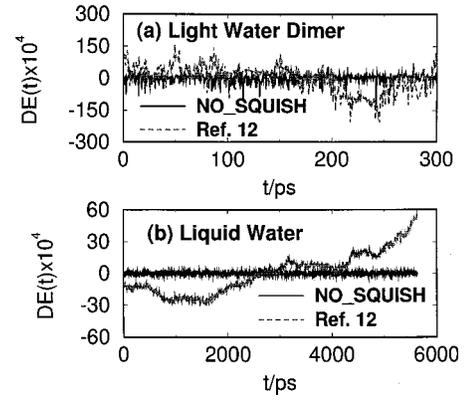
FIG. 2. (a) Light water dimer ( $m_H = 0.1$  amu) at  $\langle T \rangle = 155$  K,  $\Delta t = 0.3$  fs. The energy conservation measure,  $DE(t) = [E(t) - \bar{E}] / |\bar{E}|$ , for NO\_SQUISH (solid line) and Ref. 12 (dotted line). (b) Liquid water at  $\langle T \rangle = 295$  K,  $\rho = 1$  g/cm<sup>3</sup> ( $m_H = 1.008$  amu),  $\Delta t = 3.0$  fs. NO\_SQUISH (solid line) and Ref. 12 (dotted line).
