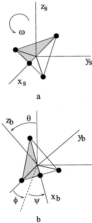
FIG. 1. (a) Angular velocity,  $\omega$ , rotates the body-fixed coordinate frame  $(x_b, y_b, z_b)$  away from the system frame  $(x_s, y_s, z_s)$ . (b) Resulting rotation is specified by the Euler angles  $(\phi, \theta, \psi)$ . Angle  $\phi$  is a counterclockwise rotation about the  $z_s$  axis. This is followed by counterclockwise rotation of  $\theta$  about the newly generated  $x$  axis shown as a dotted line. Last,  $\psi$  is a rotation about the newly generated  $z$  axis.
