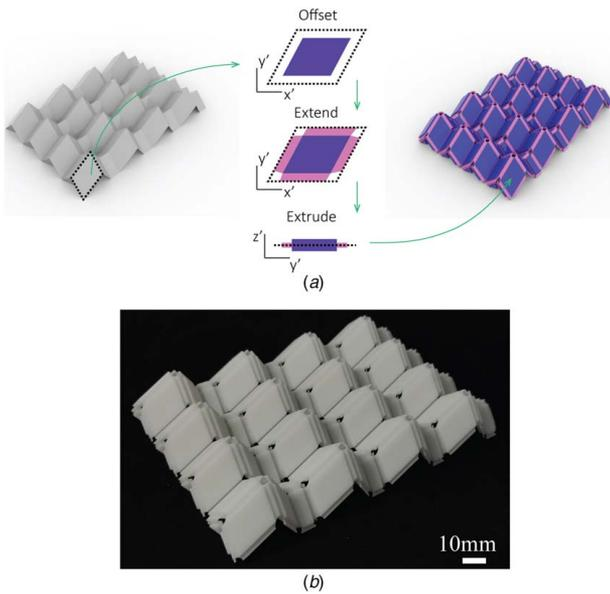
**Fig. 14 Shrimp pattern by 3D printing. (a) Procedure to prepare 3D printable solid from geometric data of a Shrimp origami surface. (b) A 3D printed Shrimp pattern using the selective laser sintering (SLS) technology. The sample shown in (b) is printed by SLS technology using a rubbery TPU material.**
