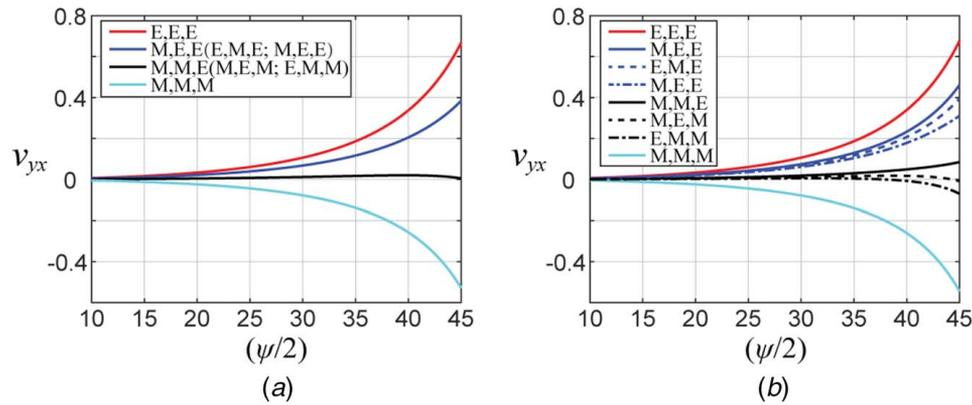
**Fig. 10 Property of the Shrimp tessellated material at different phases. (a) Poisson's ratio at different phases of variant (1). Note that some phases share the same property. (b) Poisson's ratio at different phases of variant (3). All phases have different properties.**
