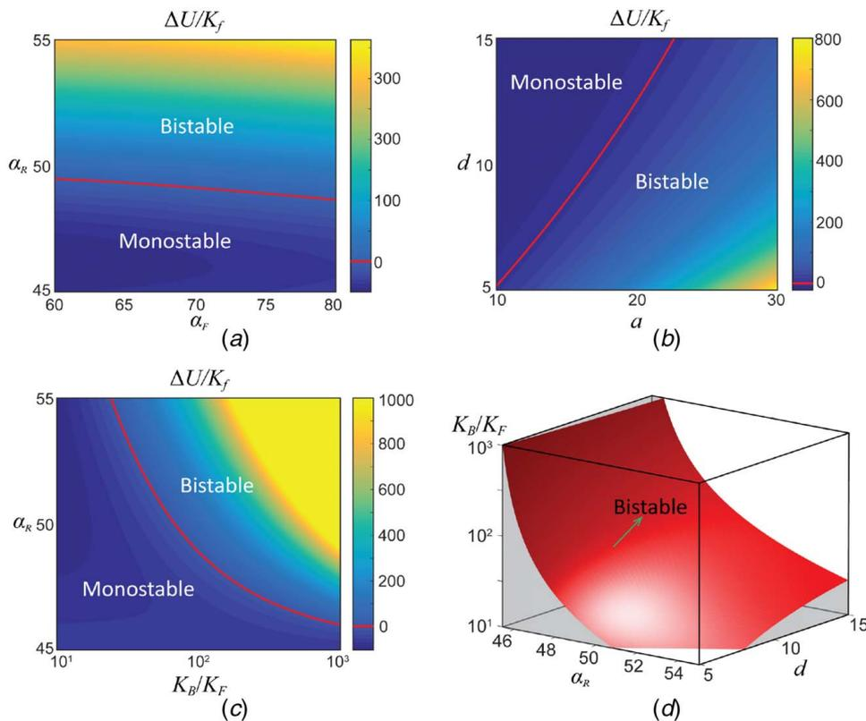
**Fig. 7 Programmable energy state of a shrimp unit cell. A positive energy difference  $\Delta U$  indicates that the pattern is bistable. (a)–(c) Show how  $\Delta U$  is affected by geometric parameters (i.e.,  $\alpha_f$ ,  $\alpha_R$ ,  $a$ ,  $d$ ) and material properties (i.e.,  $k_0^B/k_0^F$ ). In (d), we plot the limit surface of the emergence of bistability in the configuration space spanned by  $\alpha_R$ ,  $d$ ,  $k_0^B/k_0^F$ .**
