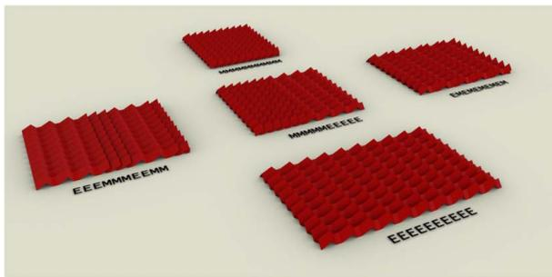
**Fig. 11 Examples of different metastable phases obtained from a single piece of Shrimp tessellated material. The text next to each configuration encodes its phase.**
