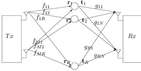
Fig. 1. Wireless relay network with several antennas at both the transmitter and receiver.
