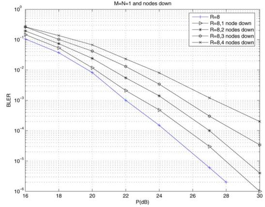
Fig. 9. For  $M = N = 1$  transmit and receive antennas, comparison of the BLER for  $R = 8$  relays if  $d = 1, 2, 3, 4$  nodes do not transmit.
