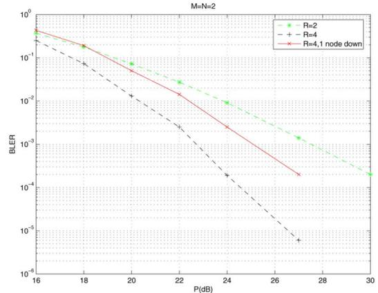
Fig. 11. For  $M = N = 2$  transmit and receive antennas, comparison of the BLER for  $R = 2$ ,  $R = 4$  relays, and  $R = 4$  relays with one node down.
