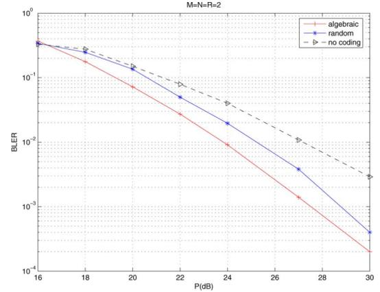
Fig. 6. For  $M = N = 2$  transmit and receive antennas,  $R = 2$  relays, the BLER of random coding is compared to the proposed algebraic construction.
