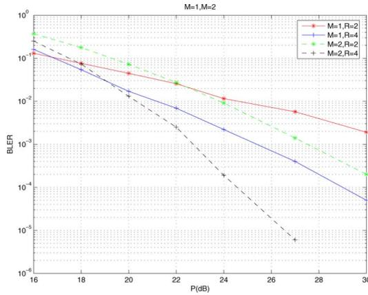
Fig. 8. For  $M = N = 2$  transmit and receive antennas, comparison of the BLER for  $R = 2$  and  $R = 4$  relays.
