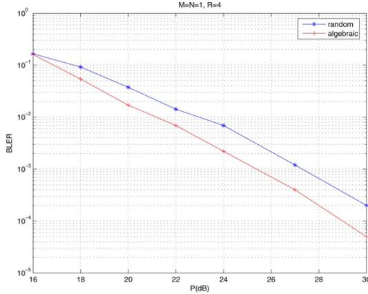
Fig. 5. For  $M = N = 1$  transmit and receive antennas,  $R = 4$  relays, the BLER of random coding is compared to the proposed algebraic construction.
