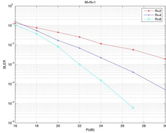
Fig. 7. For  $M = N = 1$  transmit and receive antennas, comparison of the BLER for  $R = 2$ ,  $R = 4$ , and  $R = 8$  relays.
