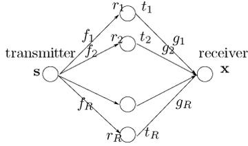
Fig. 4. Wireless network with a single antenna at the transmitter and receiver.
