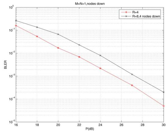
Fig. 10. For  $M = N = 1$  transmit and receive antennas, comparison of the BLER for  $R = 4$  relays and  $R = 8$  relays with half of them down.
