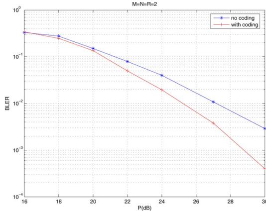
Fig. 3. For  $M = N = 2$  transmit and receive antennas,  $R = 2$  relays, comparison of the BLER with and without coding at the transmitter. Random coding is used at the relays. We see a clear loss in the diversity when no coding is used at the transmitter.
