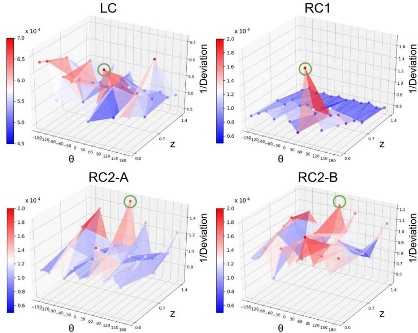
**Fig. SI-2: Deviation plots.** Total 36 electrode placements were tested in the simulation models. The deviations between the simulated impedance and experimental impedance at 10 kHz were calculated and the best fit scenario of electrode position is highlighted in the green circle.
