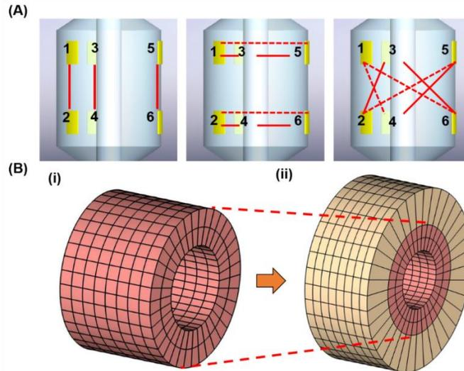
**Fig. SI-5: Finite element model for reconstructing the conductivity maps.** (A) The configuration of the 6-point electrodes (EIS sensor) generates 15 permutations. (B-i) 576-element mapping scheme represents the inner smooth muscle layer. (B-ii) 864-element mapping scheme includes the collagen layer (yellow).
