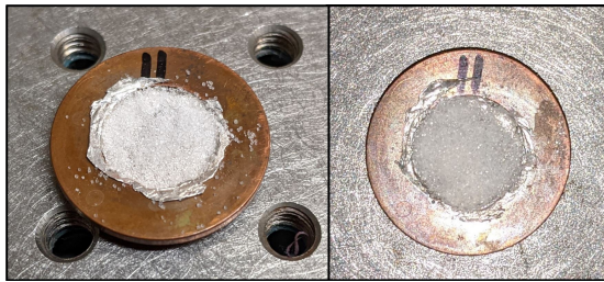
Figure 3. The sodium chloride sample after pressing into indium foil and pouring off non-attached grains. The surface area of the sample predominantly shows sodium chloride grains, though in the specular image on the right reflection can be seen from some small regions of bare indium.
