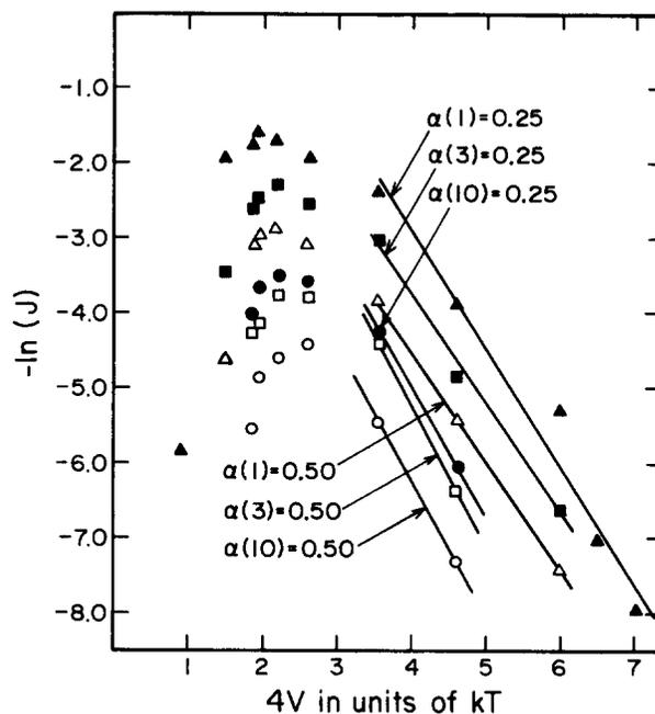
FIG. 2. Semilogarithmic graph of jumps per atom ( $J$ ) required to attain Warren SRO parameters:  $\alpha(1) = 0.25$ ,  $\alpha(3) = 0.25$ ,  $\alpha(10) = 0.25$ ,  $\alpha(1) = 0.5$ ,  $\alpha(3) = 0.5$ , and  $\alpha(10) = 0.5$ , vs  $4V$ . Vacancy mechanism with  $U = 0$ . Lines were least squares fit to the low temperature data.
