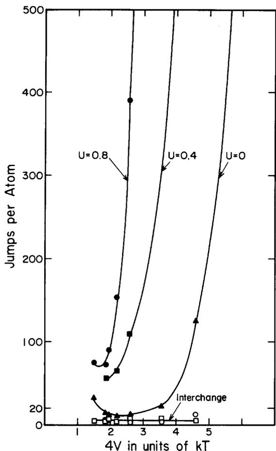
FIG. 1. Number of average jumps per atom required to attain a Warren SRO parameter,  $\alpha(1) = 0.25$ , vs  $4V$ . Interchange mechanisms and the vacancy mechanism with  $U = 0$ ,  $U = 0.4$ , and  $U = 0.8$ . Lines were drawn to guide the eye.
