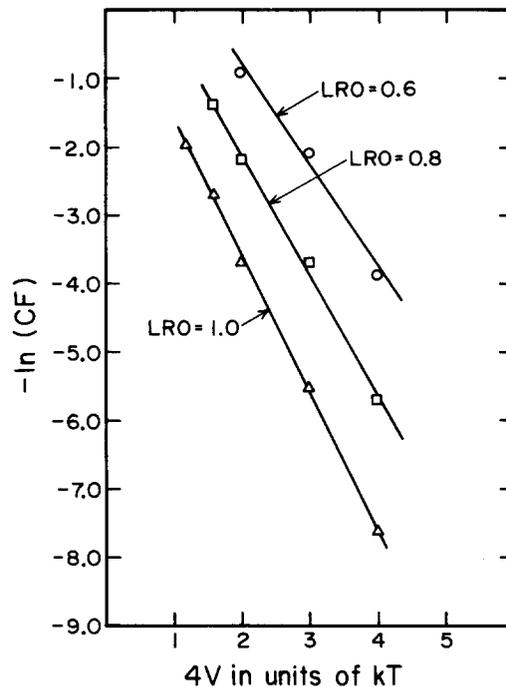
FIG. 5. Semilogarithmic graph of the Beeler and Delaney contraction factor (CF) (Ref. 14) vs  $4V$ . For  $10^6$  jumps of the vacancy and initial long range order (LRO) of 0.6 (top), 0.8 (middle), and 1.0 (bottom). Lines were least squares fit to the data.
