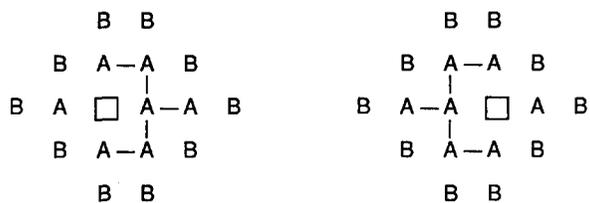
FIG. 6. A pair of local lattice arrangements which comprise a strong vacancy trap when  $V_A$  is large and  $U = 1$ .
