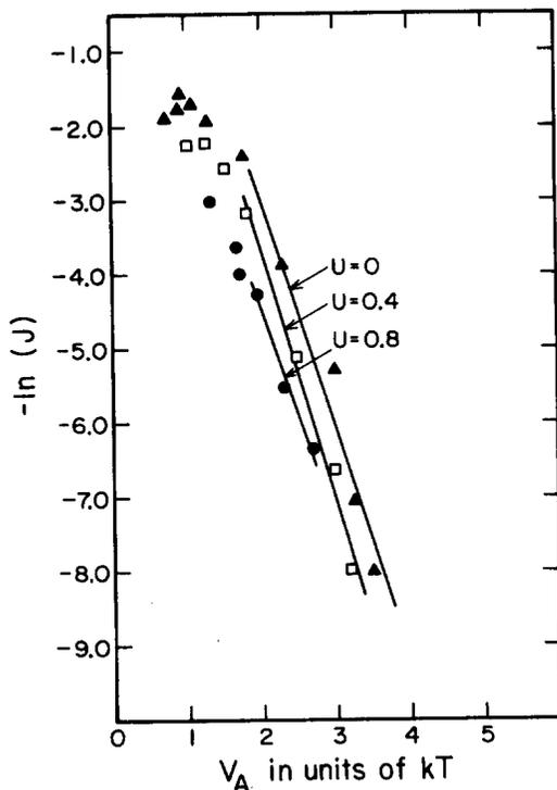
FIG. 4. Semilogarithmic graph of jumps per atom ( $J$ ) required to attain a Warren SRO parameter,  $\alpha(1) = 0.25$ , vs  $V_A$ . Vacancy mechanism with  $U = 0$ ,  $U = 0.4$ , and  $U = 0.8$ . Lines were least squares fit to the low temperature data.
