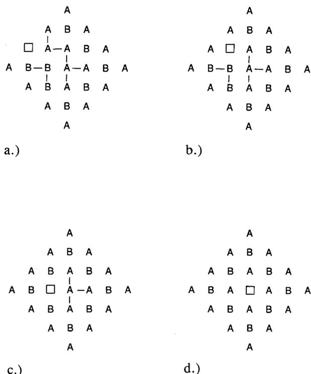
FIG. 8. A vacancy trap in a region of mostly ordered lattice: (a) an entry site, (b) an intermediate site, (c) and (d) sites of strongest trapping.
