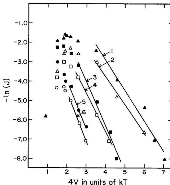
FIG. 3. Semilogarithmic graph of jumps per atom ( $J$ ) required to attain specific Warren SRO parameters vs  $4V$ . Vacancy mechanism. Curve (1)  $\alpha(1) = 0.25$ ,  $U = 0$ ; (2)  $\alpha(3) = 0.25$ ,  $U = 0$ ; (3)  $\alpha(1) = 0.25$ ,  $U = 0.4$ ; (4)  $\alpha(3) = 0.25$ ,  $U = 0.4$ ; (5)  $\alpha(1) = 0.25$ ,  $U = 0.8$ ; (6)  $\alpha(3) = 0.25$ ,  $U = 0.8$ . Lines were least squares fit to the low temperature data.
