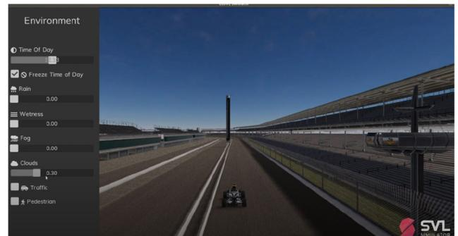
FIGURE 11. FITENTH vehicle in the SVL simulator [75] on a 1:10 scale version of the Indianapolis Motor Speedway.
