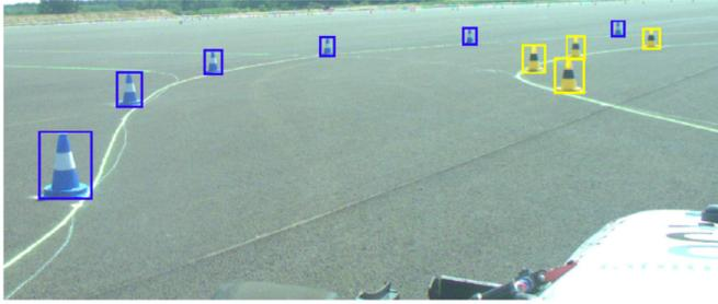
**FIGURE 3.** Exemplary cone detection in the Formula Student Driverless competition. The racetrack is defined by a left boundary (blue cones) and a right boundary (yellow cones) which need to be detected by the teams. This image is part of the FSOCCO dataset [49] that supports FSD teams with the development of their perception pipelines.
