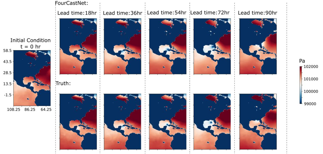
Figure 11: FourCastNet Predictions of the Mean Sea-Level Pressure with the corresponding ground truth at Forecast lead times of up to 72 hours. The forecast was initialized at a calendar time of October 7, 2018 00:00 UTC. A land-sea mask was applied to make the MSLP zero over landmass for better visualization.
