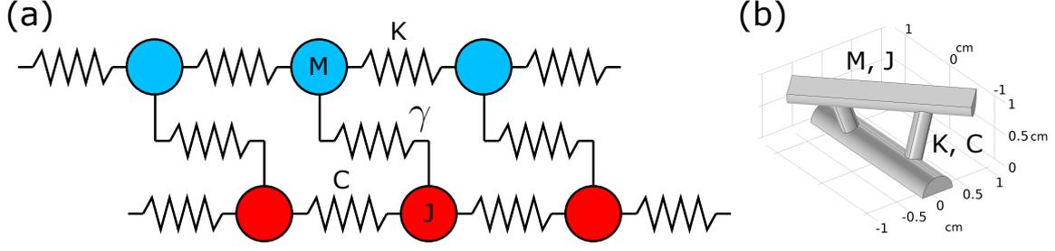
Figure S1: (Color Online) (a) A ladder-like meta chain model with a mass  $M$ , stiffness  $K$ , moment of inertia  $J$ , torsional rigidity  $C$ , and coupling stiffness  $\gamma$ . (b) A representative volume element of the HMMs used for the analytical model.
