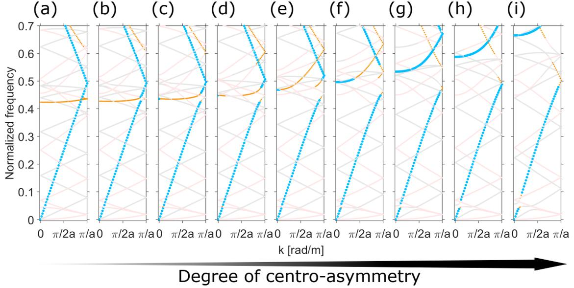
Figure S2: (Color Online) Dispersion curves of the HMMs with increasing degree of centro-asymetry: (a) 50-50 (centrosymmetric), (b) 43.25-56.25, (c) 37.5-62.5, (d) 31.25-68.75, (e) 25-75, (f) 18.75-81.25, (g) 12.5-87.5, (h) 6.25-93.75, and (i) 0-100 (fully centro-asymetric) material distribution. The longitudinal modes (blue) and the transitional modes (orange) are highlighted to show the evolution of longitudinal band gaps.
