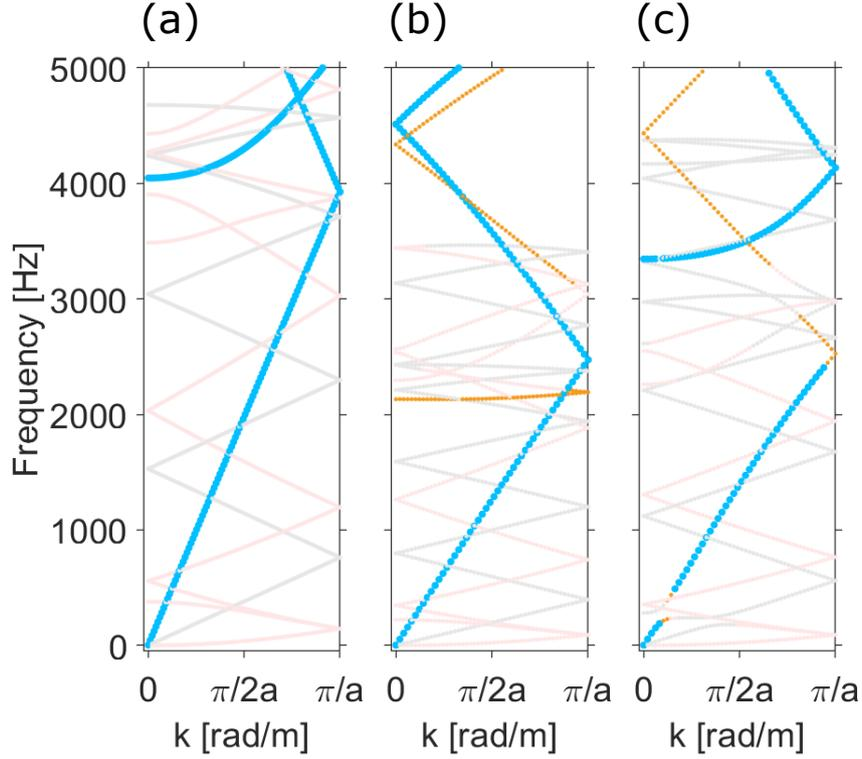
Figure S3: (Color Online) Dispersion curves of the (a) centrosymmetric HMMs with same material inserts as the base material, (b) centrosymmetric HMMs with heavier stainless steel inserts, and (c) fully centro-asymmetric HMMs with heavier stainless steel inserts. The longitudinal modes (blue) and the transitional modes (orange) are highlighted to show the evolution of longitudinal band gaps. The color of the torsional mode (black) and the rotaional modes (red) are suppressed in the background.
