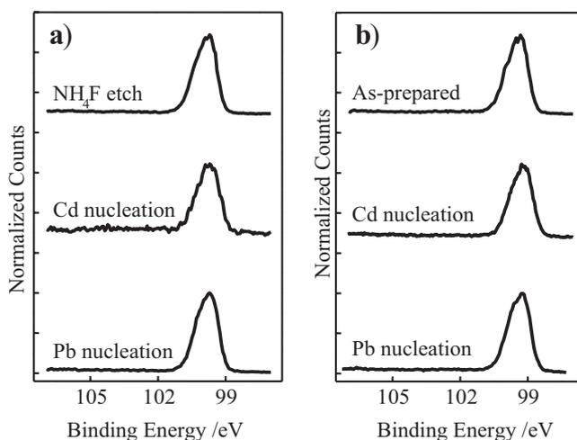
**Figure 5.** X-ray photoelectron spectra of the Si 2p region of (a) H-terminated and (b)  $\text{CH}_3$ -terminated  $n$ -Si(111) electrode surfaces (top) as-prepared, (middle) after initial Cd nucleation step, and (bottom) after initial Pb nucleation step.
