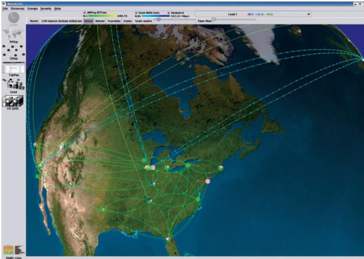
**Figure 2.** The MonAlisa framework. MonAlisa provides a distributed monitoring service system in which each station server hosts and can schedule many dynamic services. It thereby acts as a dynamic service system that can be discovered and used by any other services or clients requiring such information.
