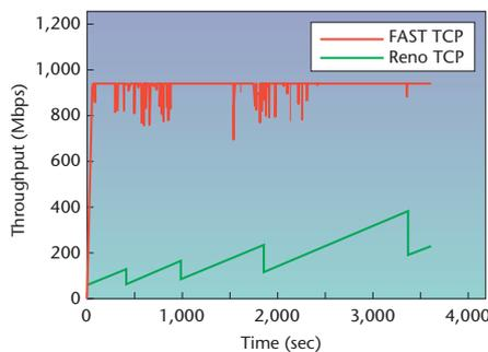
**Figure 3.** Throughput of FAST TCP flows compared with Reno in the presence of packet loss. FAST TCP stabilizes at a steady high throughput whereas Reno ramps up much slower at a lower throughput.
