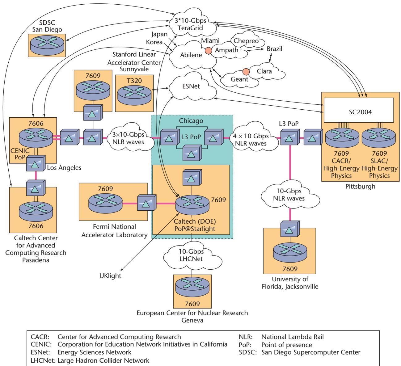
**Figure 4. High-speed terabyte transfers for physics demonstration at Supercomputing 2004. Using FAST TCP and links provided by various organizations, we achieved an aggregate rate of 101 Gbps to and from the conference floor.**
