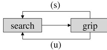
Figure 6. Macroscopic state diagram of the multirobot system. The arrow marked “s” corresponds to the transition from the gripping to the searching state after a successful collaboration, while the arrow marked “u” corresponds to the transition after an unsuccessful collaboration, that is, when the robots time out.
