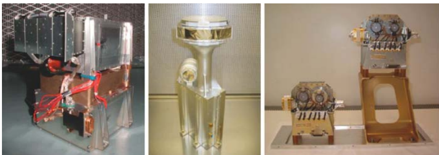
Fig. 10 The SEP instrument suite of STEREO, from left to right, SIT, HET/LET, and SEP [17]
