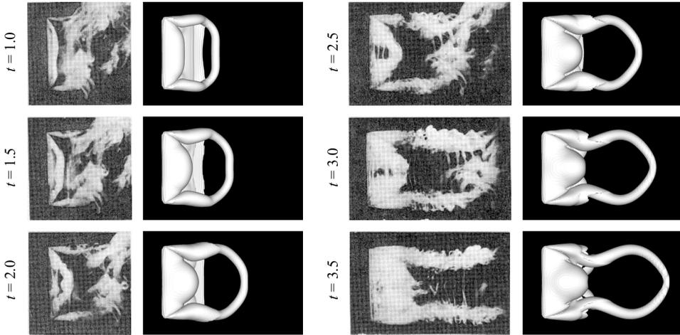
FIGURE 5. Top views of the wake vortices behind a rectangular wing of  $AR=2$  at  $\alpha=40^\circ$  from smoke visualizations at  $Re_a=5200$  and present results at  $Re=500$  with iso-contour of  $\|\omega\|_2=5$ . Smoke visualizations are from Freymuth *et al.* (1987); reprinted by permission of the American Institute of Aeronautics and Astronautics.
