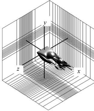
FIGURE 1. A typical computational domain showing the top-port side of the wake around a rectangular flat plate of  $AR=2$ . The spatial discretization of this computational domain is shown for every five cells for the  $x$ - and  $y$ -directions and four cells for the  $z$ -direction.
