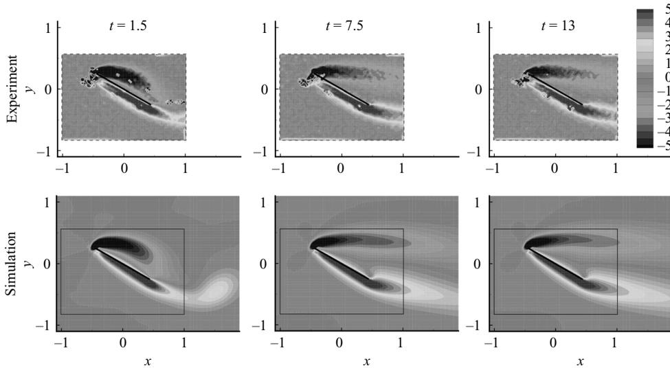
FIGURE 2. Snapshots of spanwise vorticity field at mid-span around a plate of  $AR=2$  at  $\alpha=30^\circ$  from the experiment and the simulation. Free stream is directed from left to right and the position of the plate is illustrated with the black solid line (for the experiment, the position is approximate due to the deflection of the plate). The boxed regions in the simulated results represent the fields of view for the DPIV measurements.
