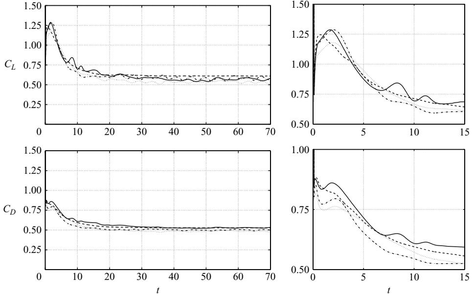
FIGURE 13. Time trace of lift and drag coefficients for rectangular (—), elliptic (⋯⋯⋯), semicircular (---) and delta-shaped (-·-·-) planforms at  $Re = 300$  and  $\alpha = 30^\circ$ . The figures on the right side magnify the corresponding (early-time) transient behaviour shown in the left-side figures.
