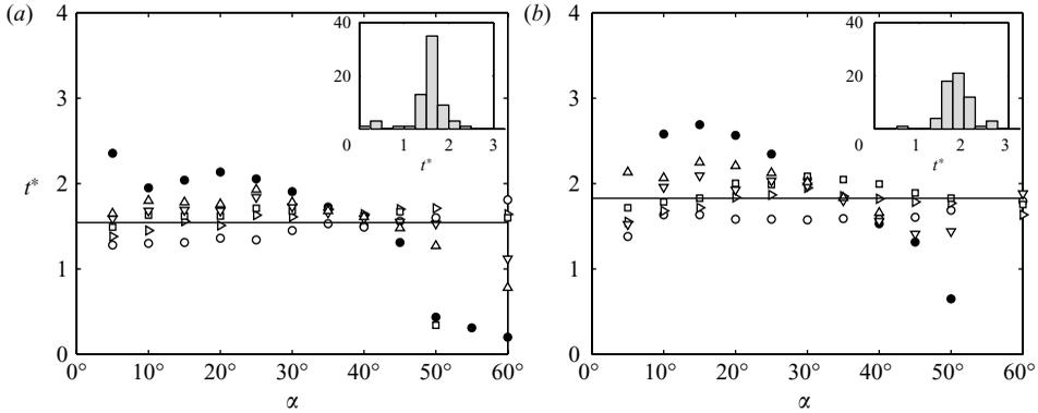
FIGURE 8. Time at which lift achieves the maximum,  $t^*$ , after an impulsive start for different angles of attack at (a)  $Re = 300$  and (b)  $Re = 500$ . Symbols denote cases for  $AR = 1$  ( $\circ$ ),  $AR = 1.5$  ( $\diamond$ ),  $AR = 2$  ( $\square$ ),  $AR = 3$  ( $\nabla$ ),  $AR = 4$  ( $\triangle$ ) and two-dimensional ( $\bullet$ ). The mean averages are shown with solid lines. The inset figures are the corresponding histograms.
