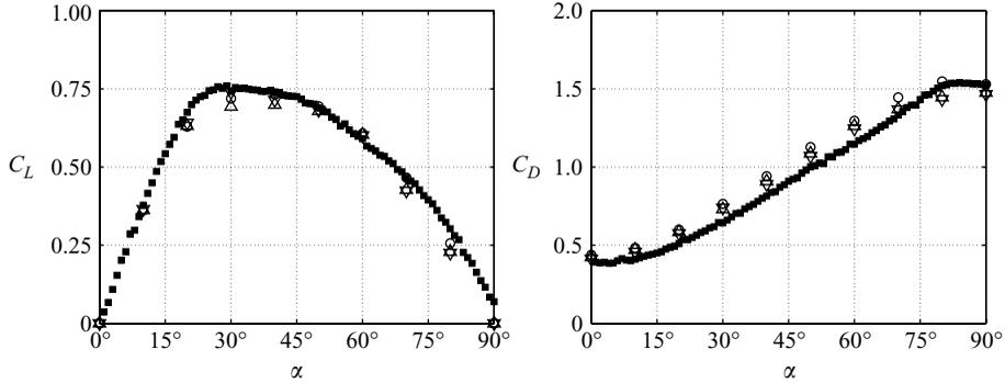
FIGURE 3. Lift and drag coefficients for a rectangular plate of  $AR=2$  at  $Re=100$ . Data from the oil tow tank experiments are shown with (■) and results from numerical simulations are presented with (○), (△) and (▽) for grid sizes of  $125 \times 55 \times 80$ ,  $150 \times 66 \times 96$  and  $200 \times 88 \times 128$ , respectively.
