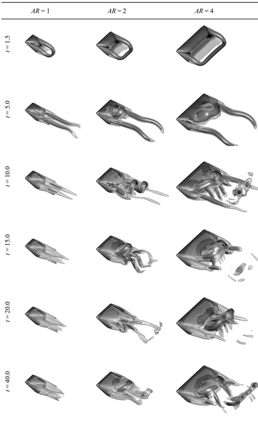
FIGURE 4. Top-port views of the wake vortices behind rectangular plates of  $AR = 1, 2$  and  $4$  at  $\alpha = 30^\circ$  and  $Re = 300$ . Shown are the iso-surface of  $\|\boldsymbol{\omega}\|_2 = 3$  in light grey with vortex cores highlighted by the iso-surface of  $Q = 3$  in dark grey.
