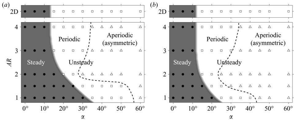
FIGURE 10. Stability of the wake for a range of  $\alpha$  and  $AR$  at (a)  $Re = 300$  and (b)  $Re = 500$ . Symbols (●), (□) and (△) denote steady, unsteady periodic and unsteady aperiodic wakes at large time. The shaded area and the dashed line approximately represent the region of stability and the transition from periodic to aperiodic shedding, respectively. Shown at the top are the two-dimensional findings.
