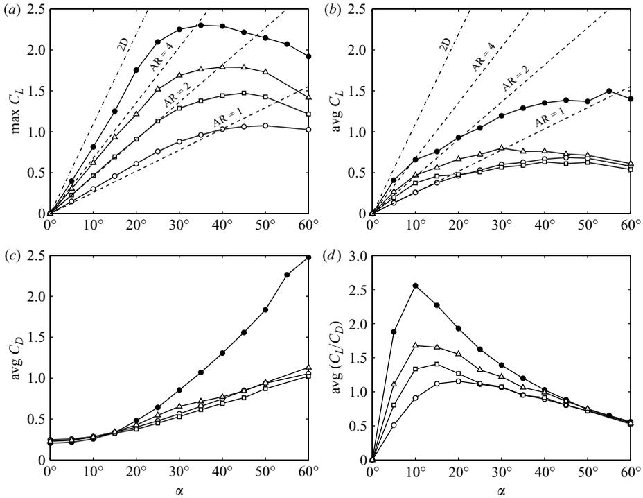
FIGURE 7. Characteristic coefficients for rectangular plates at  $Re = 300$ : (a) maximum lift; (b) time-averaged lift coefficient at large time; (c) time-averaged drag coefficient at large time and (d) time-averaged lift-to-drag ratio at large time for  $AR = 1$  ( $\circ$ ),  $AR = 2$  ( $\square$ ),  $AR = 4$  ( $\triangle$ ) and two-dimensional ( $\bullet$ ). Overlaid are the two- (—) and three-dimensional (----) inviscid lift limits.
