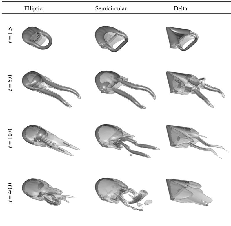
FIGURE 12. Top-port views of the wake vortices behind different planform geometries at  $\alpha = 30^\circ$  and  $Re = 300$  with the iso-surface of  $\|\boldsymbol{\omega}\|_2 = 3$  in light grey with vortex cores highlighted by the iso-surface of  $Q = 3$  in dark grey.
