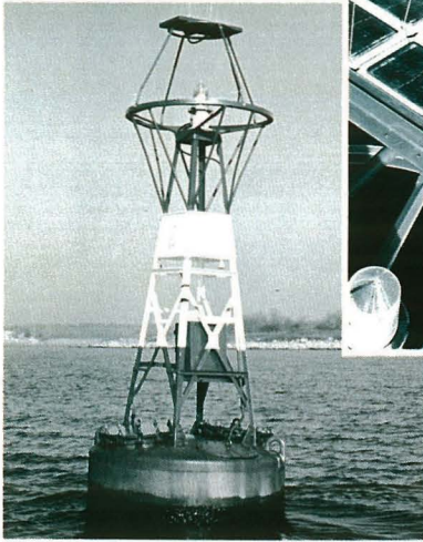
U.S. Coast Guard buoy with photovoltaic-powered navigational light.
