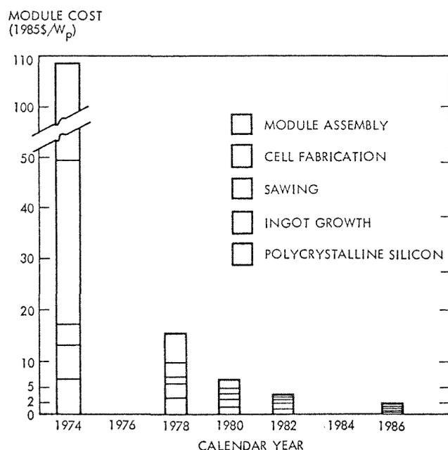
Figure 7. State-of-the-Art Projections for Czochralski Module Technology (1974 to 1985)
