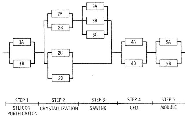
Figure 2. Task Network for Solar-Cell Module Production
