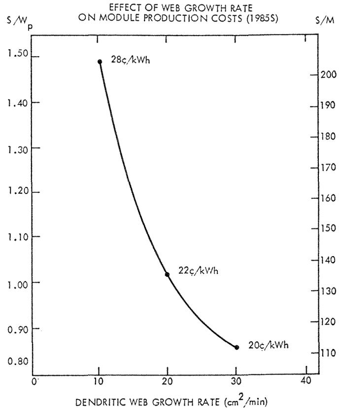
Figure 8. Effect of Web Growth-Rate on Module Production Costs (1985 dollars)
