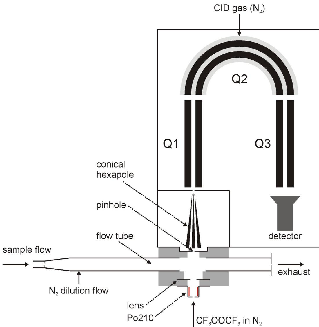
**Figure S1** Schematic diagram of the Caltech Chemical Ionization Mass Spectrometer (CIMS).
