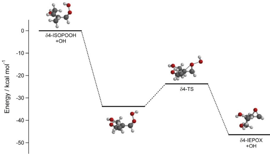
**Figure S3** Relative energies of the B3LYP/cc-pVTZ optimized geometries for the formation of  $\delta 4\text{-IEPOX}$  from  $\delta 4\text{-ISOPOOH}$ .
