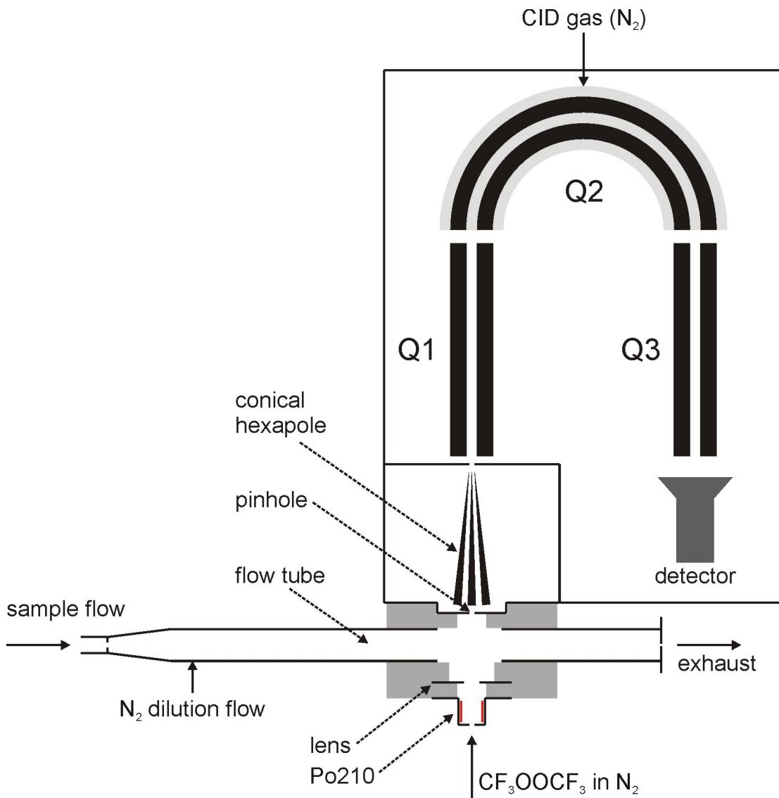
**Figure S1** Schematic diagram of the Caltech Chemical Ionization Mass Spectrometer (CIMS).
