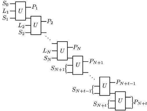
Fig. 6. Circuit diagram of a quantum convolutional encoder with seed transformation  $U$ . The superscripts indicating the number of qubits per wire are omitted for clarity, and can be found in Fig. 7.
