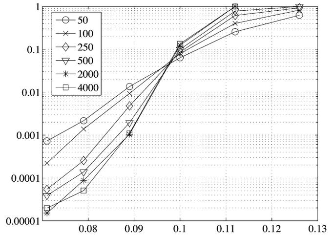
Fig. 12. WER versus depolarizing probability  $p$  for the quantum turbo code obtained from the concatenation of the convolutional code with seed transformation  $U_{(3,1,3)}$  with itself, for different number of encoded qubits  $K$ . Each constituent convolutional code has  $m = 3$  qubits of memory and has rate  $\frac{1}{3}$ , so the rate of the turbo code is  $\frac{1}{9}$ .
