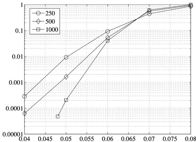
Fig. 14. WER versus depolarizing probability  $p$  for the quantum turbo code obtained from the concatenation of the convolutional code with seed transformation  $U_{(2,1,4)}$  with itself, for different number of encoded qubits  $K$ . Each constituent convolutional code has  $m = 4$  qubits of memory and has rate  $\frac{1}{2}$ , so the rate of the turbo code is  $\frac{1}{4}$ .
