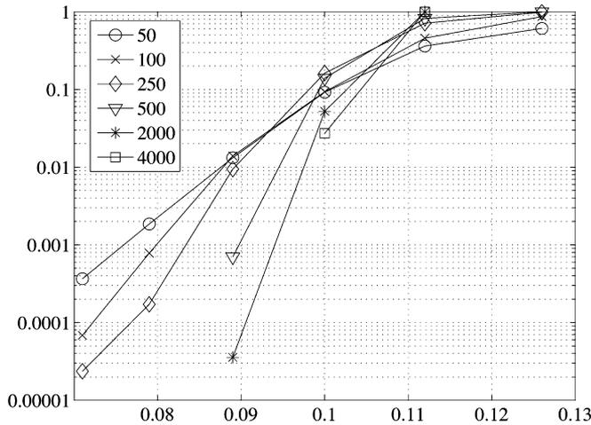
Fig. 13. WER versus depolarizing probability  $p$  for the quantum turbo code obtained from the concatenation of the convolutional code with seed transformation  $U_{(3,1,4)}$  with itself, for different number of encoded qubits  $K$ . Each constituent convolutional code has  $m = 4$  qubits of memory and has rate  $\frac{1}{3}$ , so the rate of the turbo code is  $\frac{1}{9}$ .
