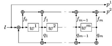
Fig. 3. Representation of convolutional encoder as a linear filter. The labels  $f$  and  $q$  take values 0 and 1 and indicate, respectively, the absence or presence of the associated wire. Although linear, this transformation is not invertible.
