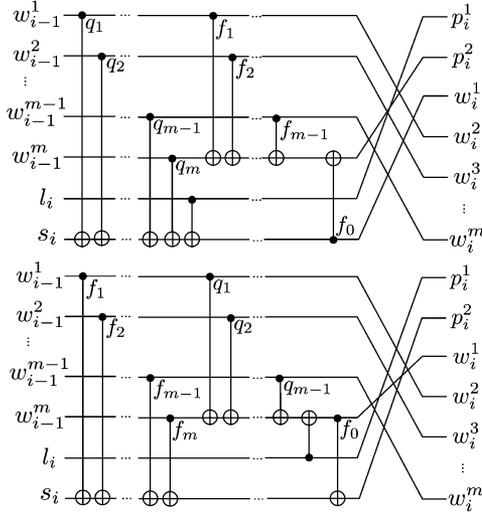
Fig. 4. Seed transformation circuit for convolutional code of Fig. 3. Top: Case  $f_m = 1$ . Bottom: Case  $q_m = 1$ . The labels  $f$  and  $q$  take values 0 and 1 and indicate, respectively, the absence or presence of the associated gate. Both circuits are entirely built from controlled nots, and are, therefore, invertible. As its name indicates, the controlled not acts by negating the target bit  $\oplus$  if and only if the control bit  $\bullet$  is in state 1.
