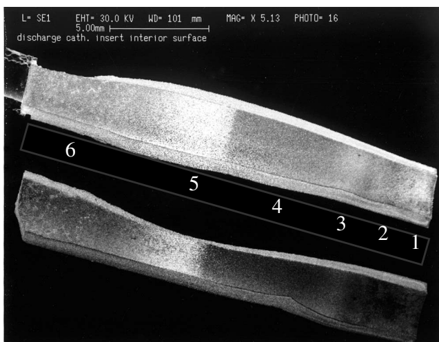
FIG. 5. Six zones on the interior of the discharge cathode insert.
