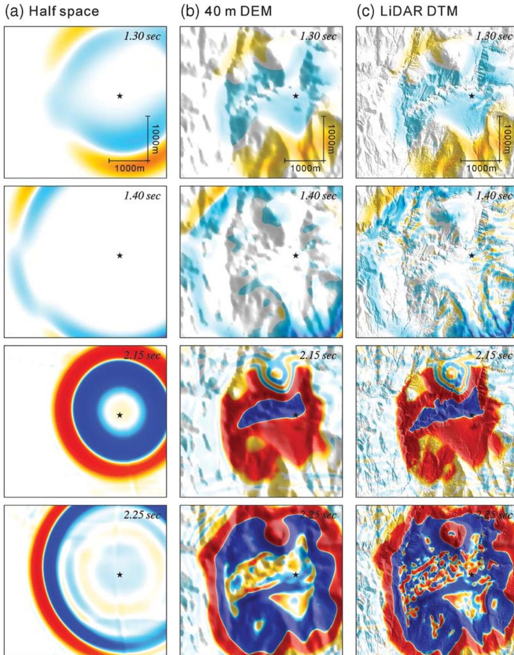
**Figure 5.** Snapshots of the north component of the wave field for three models: (a) 3D wave-speed model with a flat ground surface, (b) 3D wave-speed model with 40 m DEM topography, and (c) 3D wave-speed model incorporating LiDAR DTM. Warm colors indicate positive values and cold colors indicate negative values. The epicenter of the double-couple source is represented by a star.
