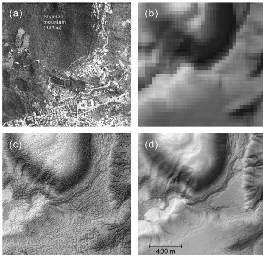
**Figure 2.** Comparative images of various topographic data sets: (a) 1/5000 aerial topographic map, (b) 40 m digital elevation model (DEM), (c)  $1 \text{ m} \times 1 \text{ m}$  LiDAR digital surface model (DSM), which includes the presence of vegetation, and (d)  $1 \text{ m} \times 1 \text{ m}$  LiDAR digital terrain model (DTM) without vegetation.
