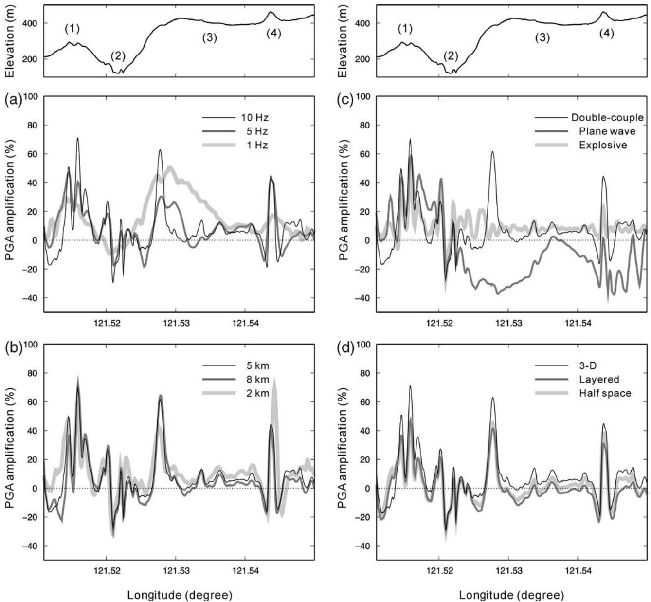
**Figure 9.** Effects due to variations in (a) source frequency, (b) source depth, (c) input wave-field type, and (d) subsurface structure by analyzing the relative change in PGA along profile A-A' in Figure 8a. The upper panels show the related cross section of the LiDAR DTM. Four specific locations are labeled by numbers along the profile.
