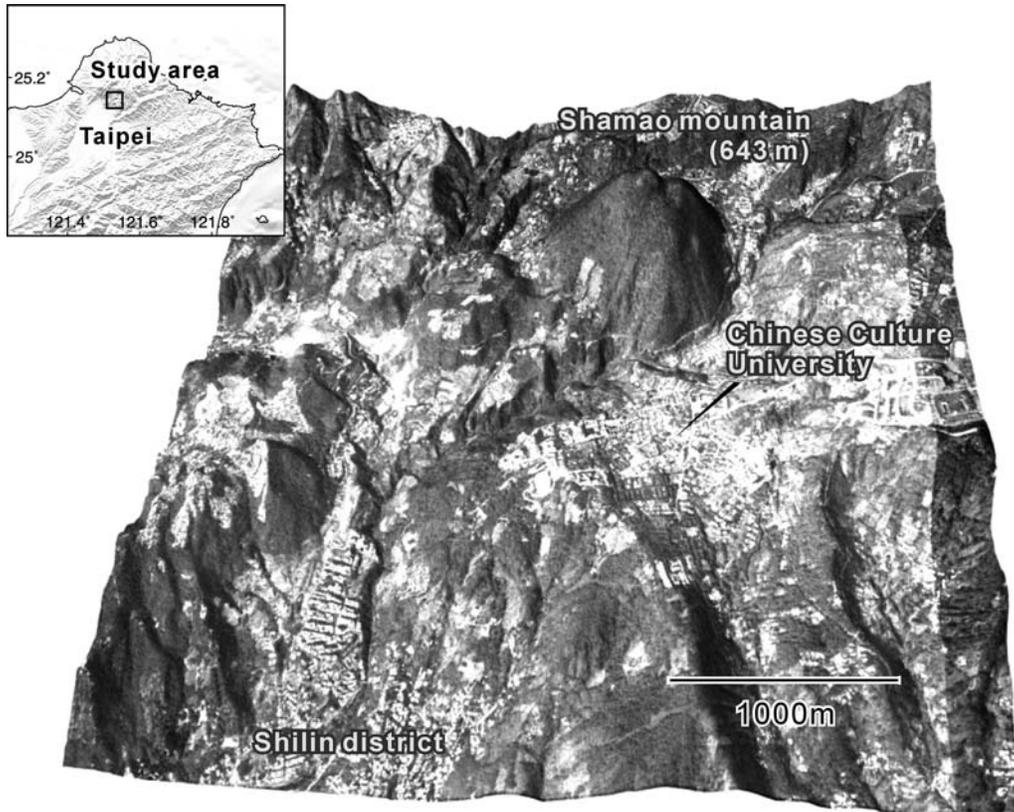
**Figure 1.** LiDAR 3D digital map of northern Taiwan. A 1/5000 aerial picture is mapped on the 1 m  $\times$  1 m LiDAR digital terrain model. The steep peak of Shamao Mountain, the high population density at the Chinese Culture University, and the Shilin district are the most striking features in the region.
