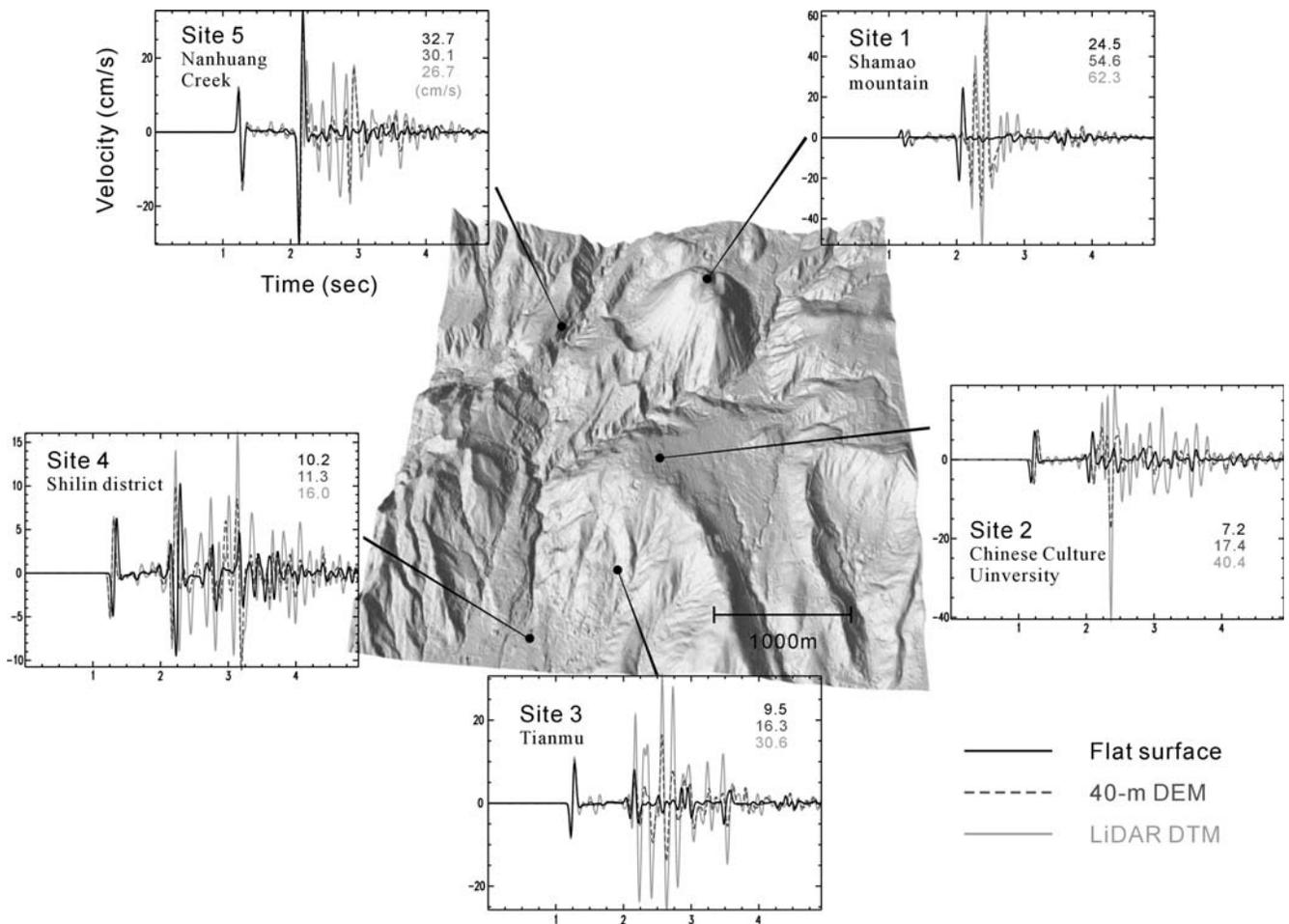
**Figure 7.** Comparison between LiDAR DTM, 40 m DEM, and flat surface synthetic waveforms at five different sites. We show the vertical component of the velocity vector, band-pass filtered between 0.1 and 10 Hz. Gray lines show the LiDAR DTM synthetic seismograms, dashed lines show the 40 m DEM synthetic seismograms, and black lines are the flat surface synthetic seismograms. Peak velocities determined for the three models are shown in the right-hand side of the figure.
