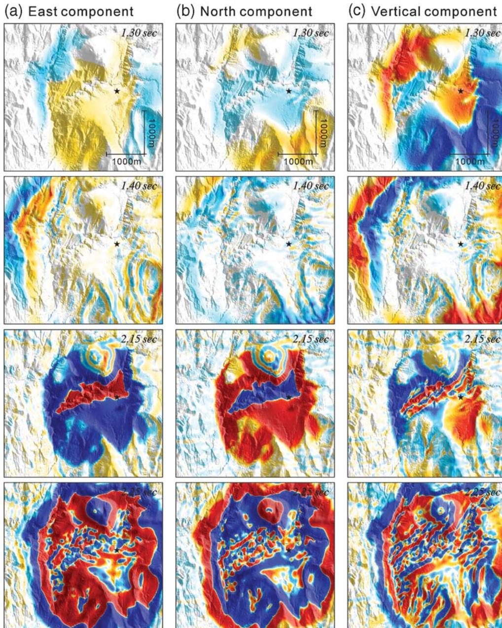
**Figure 4** Snapshots of the three components of the wave field for a simulation of a hypothetical double-couple source located beneath the study area at a depth of 4.92 km: (a) east component, (b) north component, and (c) vertical component. Warm colors indicate positive values and cold colors indicate negative values. The wavefronts are significantly distorted. They are reflected and scattered by steep topography, especially the horizontal components.
