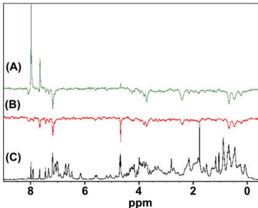
**Figure S3.** Comparison of the  $^1\text{H}\{^{19}\text{F}\}$  NOE upon selective inversion of bound and free  $^{19}\text{F}$  signal. A) Selective inversion of bound ligand. B) Selective inversion of free ligand. C) 1-D  $^1\text{H}$  NMR spectrum.
