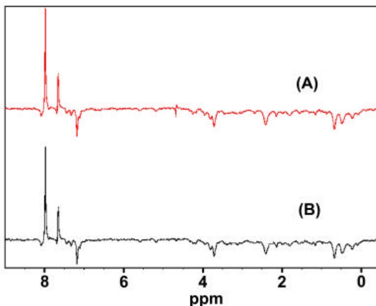
**Figure S1.**  $^1\text{H}\{^{19}\text{F}\}$  NOE spectra recorded using different recycle delays A) 8 s, B) 3.5 s.
