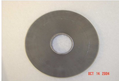
FIGURE 3. A Finemet core FT3M made by Hitachi.
