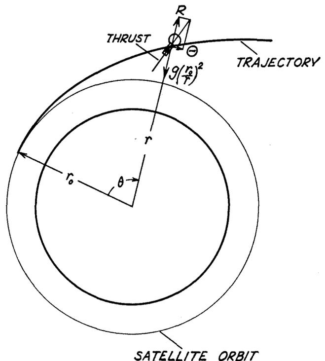
FIG. 1 TAKE-OFF FROM THE SATELLITE ORBIT WITH THRUST IN THE PLANE OF SATELLITE ORBIT
