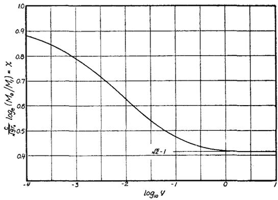
FIG. 3 MASS RATIO FACTOR  $(c/\sqrt{gr_0}) \log_e (M_0/M_1)$  AGAINST ACCELERATION FACTOR  $\nu$  FOR CIRCUMFERENTIAL THRUST.  $c$ , EFFECTIVE EXHAUST VELOCITY;  $g$ , GRAVITY AT THE SATELLITE ORBIT OF RADIUS  $r_0$ ;  $M_0$  INITIAL MASS;  $M_1$ , FINAL MASS;  $\nu$ , THE RATIO OF INSTANTANEOUS THRUST PER UNIT MASS AND  $g$  FOR CIRCUMFERENTIAL THRUST
