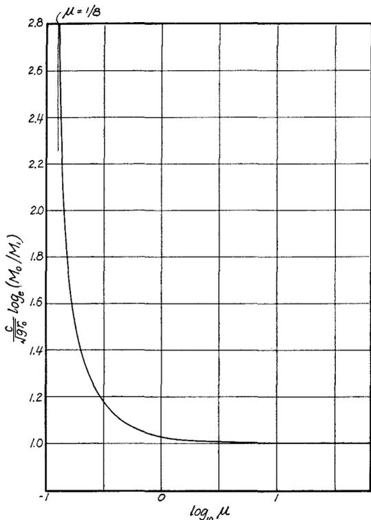
FIG. 2 MASS RATIO FACTOR  $(c/\sqrt{gr_0}) \log_e (M_0/M_1)$  AGAINST ACCELERATION FACTOR  $\mu$  FOR RADIAL THRUST.  $c$ , EFFECTIVE EXHAUST VELOCITY;  $g$ , GRAVITY AT THE SATELLITE ORBIT OF RADIUS  $r_0$ ;  $M_0$ , INITIAL MASS;  $M_1$ , FINAL MASS;  $\mu$ , THE RATIO OF INSTANTANEOUS THRUST PER UNIT MASS AND  $g$  FOR RADIAL THRUST
