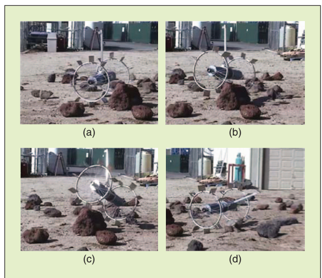
Figure 14. (a)–(d) Axel uses its large radius paddle wheels to traverse over a rock more than half of its wheel diameter in the JPL Mars Yard.
