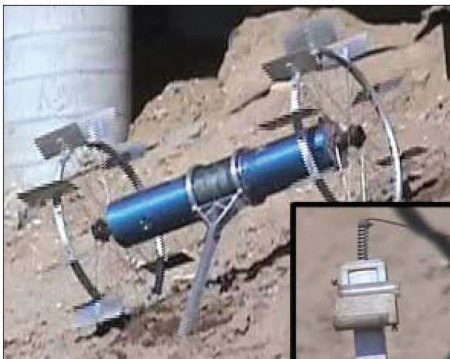
Figure 4. Axel taking a sample by pointing the caster arm into the ground and turning in place. Sand enters through the openings on the ends of the removable sampling tubes (inset).
