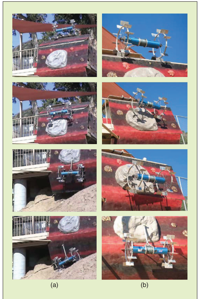
Figure 13. (a) Axel descending down onto sloped terrain in the JPL Mars Yard. (b) Axel ascending over a simulated crater promontory onto a mock lander.
