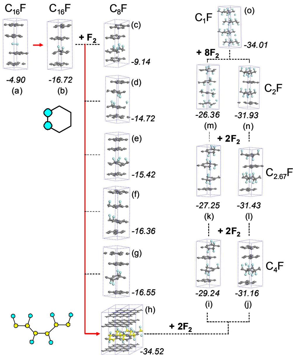
Figure S5A. The formation mechanism of graphite fluorides by the ortho configuration of fluorine. The numbers underneath the structures indicate their heat of formation (in kcal/mol) relative to pure graphite and a F<sub>2</sub> molecule, calculated by DFT. Here the final product is Fig. (h) of C<sub>8</sub>F.
