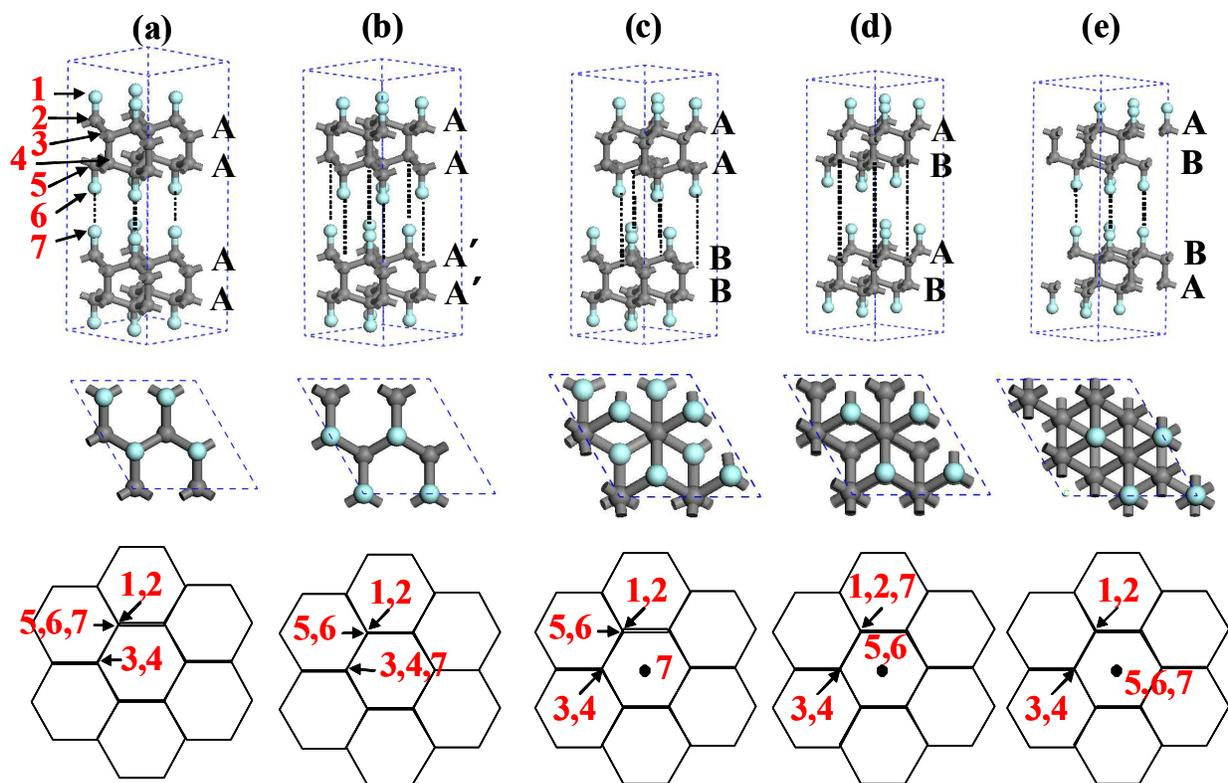
*Figure S1.* Atomic configurations of  $C_2F$  ( $CF_{0.5}$ ) crystal structures shown in Fig. 3(a)-(e). The first column indicates the overview of each structure, the second is top view, and the third is the schematic picture of atomic configuration. Here gray and cyan are carbon and fluorine, respectively. Also, the numbers of 1, 6, and 7 means fluorine atoms and 2-5 carbon atoms.
