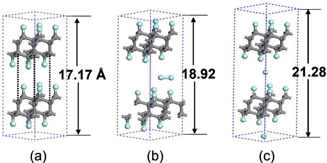
*Figure S3.* DFT results on structural change of  $C_2F$  ( $CF_{0.5}$ ) crystal (Fig. S1(d)) as proposed by Touhara et al.<sup>7</sup> with further fluorination. (a) pure  $C_2F$ , (b)  $C_2F$  after adding a  $F_2$  molecule, and (c)  $C_2F$  after adding two F atoms. These structures show the end-points of the DFT-energy minimization and indicate that no C-C bond cleavage takes place and fluorine remains in the interlayer-space.
