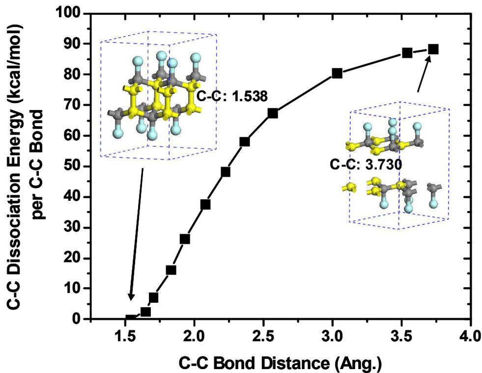
*Figure S4.* DFT results on C-C bond dissociation of  $C_2F$  ( $CF_{0.5}$ ) crystal (Fig. S1(d)) as proposed by Touhara et al.<sup>7</sup> During geometry optimization process, carbon atoms (yellow) with C-C carbon bonds are fixed, however all of others are fully optimized. And because of calculation cost, only two graphene layers were considered.
