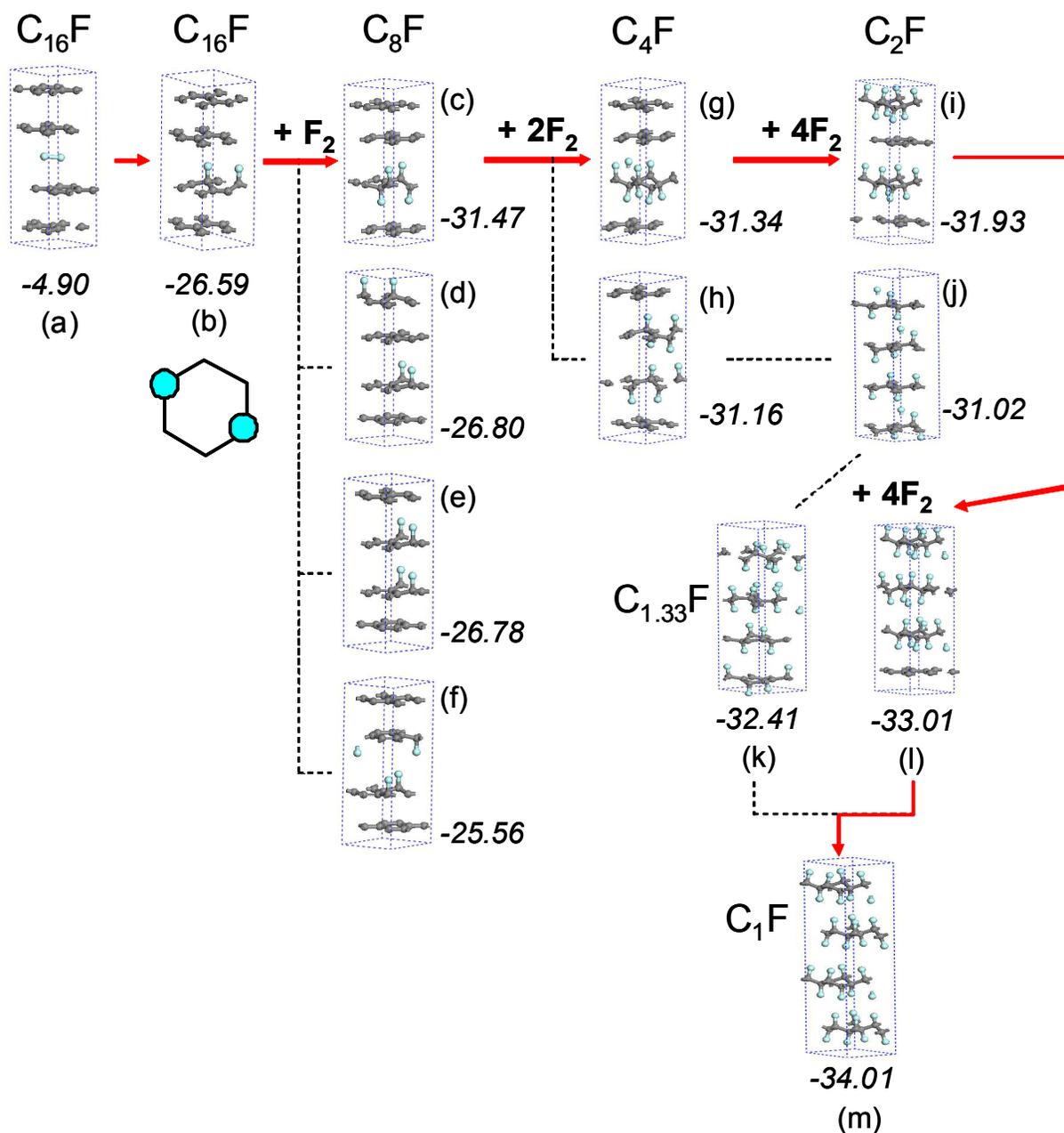
Figure S5B. The formation mechanism of graphite fluorides by the para configuration of fluorine. The numbers underneath the structures indicate their heat of formation (in kcal/mol) relative to pure graphite and a F<sub>2</sub> molecule, calculated by DFT. Here the final product is Fig. (m) of boat-type C<sub>1</sub>F, and Fig. (j) is same to a model suggested by Kita et al.<sup>9c</sup>
