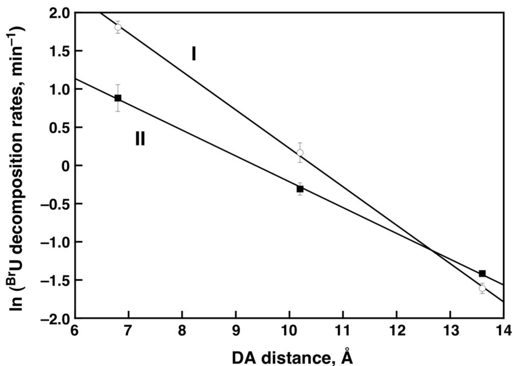
**FIGURE 5.** Initial decomposition rates ( $\text{min}^{-1}$ ) of  $\text{BrU}$  as a function of the distance between the naphthalene-modified uridine (Donor – D) and the  $\text{BrU}$  (Acceptor – A) for DNA sets I and II. Experimental conditions:  $\lambda_{\text{ex}} = 340 \text{ nm}$  (Hg-Xe lamp, 1000 W), [naphthalene-modified DNA] =  $10 \mu\text{M}$ , 50 mM TRIS-HCl pH7.4, 100 mM NaCl. Error bars are also given.
