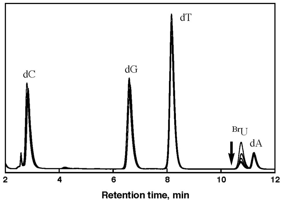
**FIGURE 3.** Overlaid HPLC chromatograms ( $\lambda_{\text{detection}} = 290$  nm) of nucleosides obtained after irradiation (0, 15, 30, 45 and 60 min,  $\lambda_{\text{ex}} = 340$  nm) and subsequent digestion of aliquots (30  $\mu\text{L}$  each) of a naphthalene-modified oligonucleotide assembly. Similar patterns are obtained for each different set of oligonucleotides.
