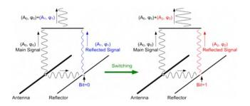
Fig. 11 Single bit modulation of the transmitted signal by digital switching the reflector in the near field.
