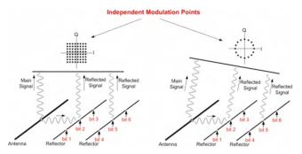
Fig. 13 Multiple reflectors with multiple switches creating different constellation points in different directions.
