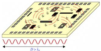
Fig. 5 Interactions between various elements on an integrated circuit above the size wavelength cross-over.
