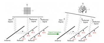
Fig. 12 Multiple reflectors with multiple switches to create different constellation points in a) the intended direction and b) in the unintended one.
