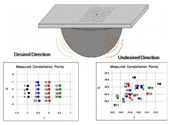
Fig. 15 The direct antenna modulation chip with a dielectric lens; a sample of the measured constellation points in the intended and unintended directions.
