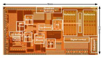
Fig. 16 The die micrograph of the direct antenna modulation transmitter.
