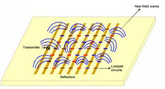
Fig. 17 A generalization of the near-field direct antenna modulation where the ports are connected to variable impedance where the nearand by extension the far field patterns can be changed continuously.
