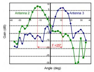
Fig. 10 Measured patterns of two adjacent antennas on a silicon chip with a backside lens.
