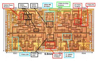
Fig. 19 Die photo of the phased-array transceiver with on-chip antennas
