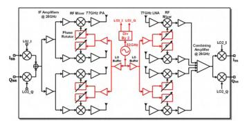
Fig. 18 The architecture of the fully-integrated 4x2 77GHz phased array transceiver with integrated antennas.
