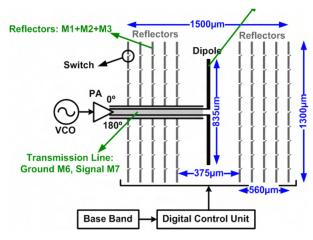
Fig. 14 The practical implementation of the digital antenna modulation scheme.
