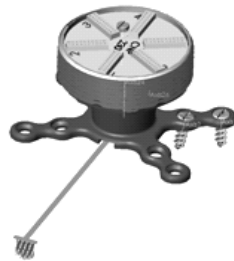
Figure 5. Schematic of the packaged silicon probes. The design shows a 96 channel device consisting of three 32 channel devices. The legs of the titanium pedestal are secured to the skull with bone screws.
