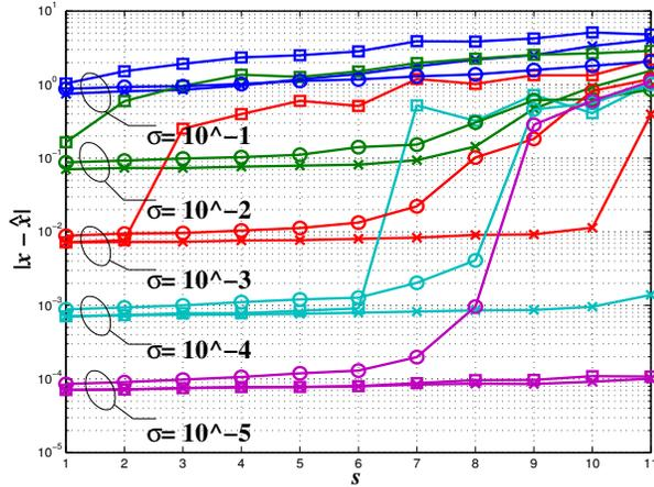
**Fig. 2.** Simulation results at different noise levels.  $N = 50$ ,  $M = 25$ ,  $\square$  is for the Berlekamp-Massey,  $\times$  is for the Coppersmith-Sudan,  $\circ$  is for the Lasso.
