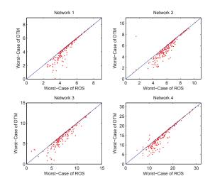
Fig. 4. Worst-case of robust optimization solution (ROS) versus worst-case of deterministic solution (DTM). For all network examples, more dots are located in the lower triangle, meaning  $z_{WC}(\mathbf{k}_{ROS}) \ge z_{WC}(\mathbf{k}_{DTM})$ .
