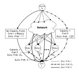
Fig. 2. One instance of robust maximum flow subgraph construction problem. All graph parameters are same as in Fig. 1 (b), except for an additional link (with no link uncertainty) between the source and the sink node.
