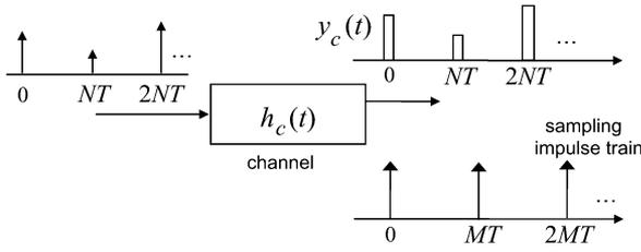
Fig. 5. Example where the system  $h_c(t)$  is a narrow pulse.
