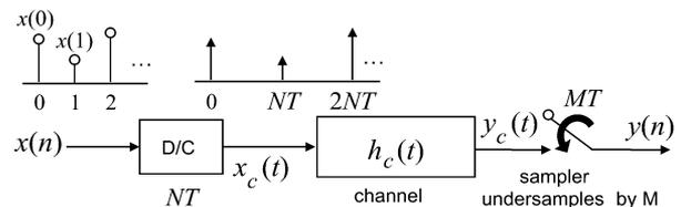
Fig. 2. Input stream transmitted at a lower rate  $1/NT$  for system identification. The receiver also performs undersampling by a factor of  $M$ .
