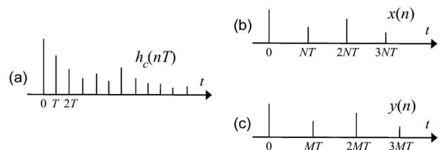
Fig. 3. Locations of (a) the channel samples at the higher rate, and (b), (c) input symbol stream and received output samples at a much lower rate.
