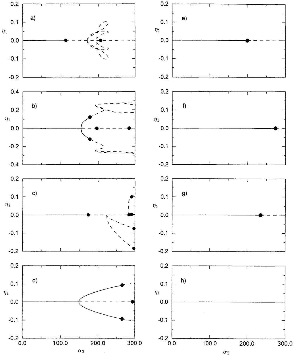
Figure 2: Maximum amplitude of  $\eta_1$  in limit cycle as a function of  $\alpha_2$  for different modal approximations,  $\bullet$ —Hopf bifurcation; a) Seven mode, b) Eight mode, c) Nine mode, d) Ten mode, e) Eleven mode, f) Twelve mode, g) Thirteen mode, h) Fourteen mode, i) Fifteen mode, j) Sixteen mode.
