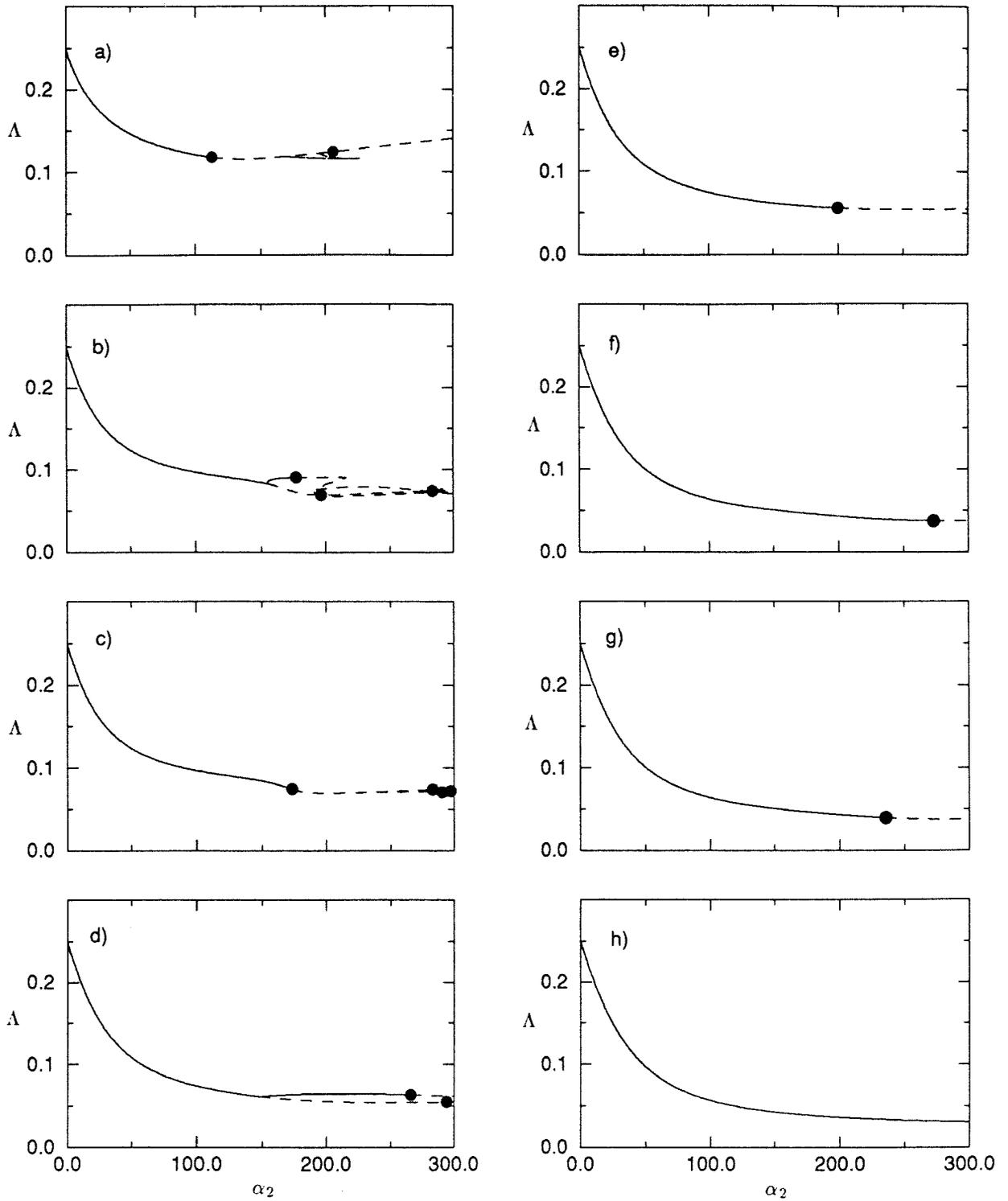
Figure 4: Ratio of linear energy production to linear energy dissipation as a function of  $\alpha_2$  for different modal approximations,  $\bullet$ —Hopf bifurcation; a) Seven mode, b) Eight mode, c) Nine mode, d) Ten mode, e) Eleven mode, f) Twelve mode, g) Thirteen mode, h) Fourteen mode, i) Fifteen mode, j) Sixteen mode.
