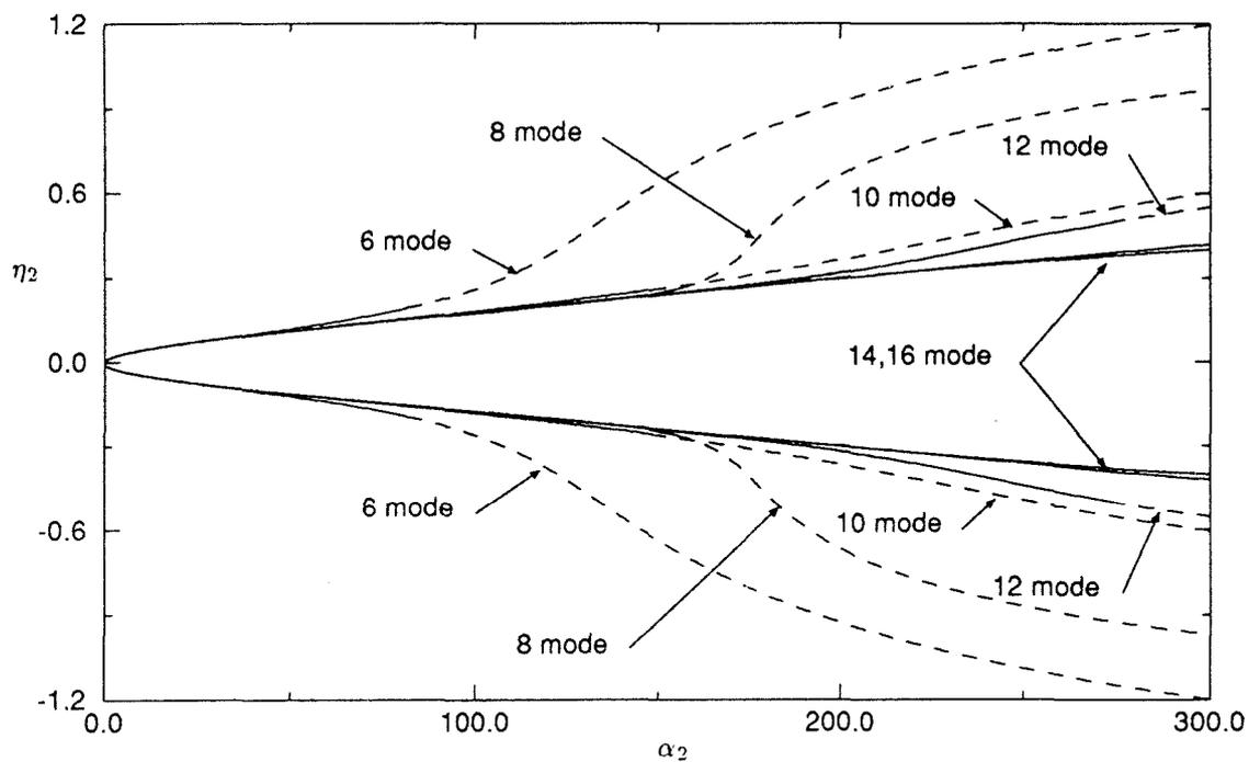
Figure 3: Maximum amplitude of  $\eta_2$  in limit cycle as a function of  $\alpha_2$  for different modal approximations.
