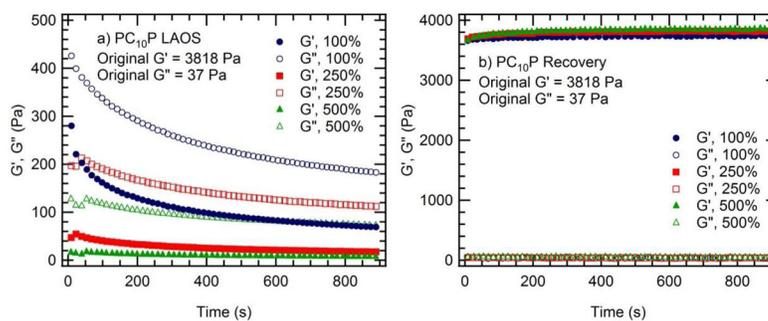
**Figure 5. Time decay and recovery of mechanical properties for PC<sub>10</sub>P under large amplitude oscillatory shear**
