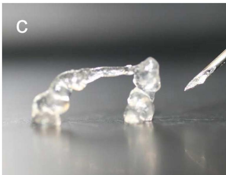
**Figure 4. Rapid recovery of hydrogels after large amplitude oscillatory strain (LAOS)**
