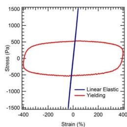
**Figure 3. Lissajous figures for PC<sub>10</sub>P**
