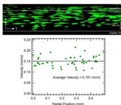
**Figure 6. Visualization of the flow profile in capillary flow of a PC<sub>10</sub>P hydrogel labeled with fluorescent microsphere tracers**
