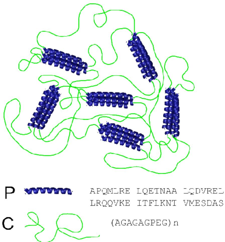
**Figure 1. Structure of telechelic protein hydrogels**
