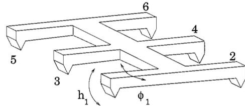
Fig. 1. Schematic of a simple hexapod robot.
