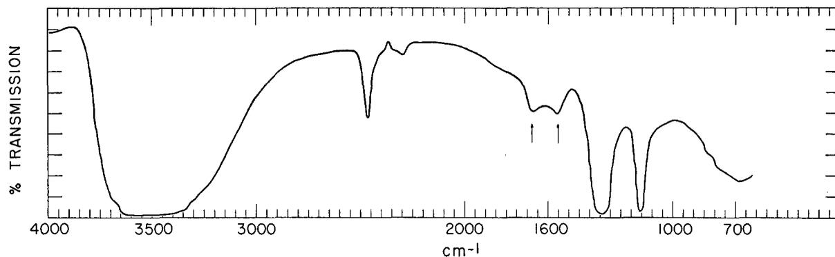
FIG. 5. Infrared spectrum of silk fibroin dissolved in a SO<sub>2</sub>-HF mixture.
