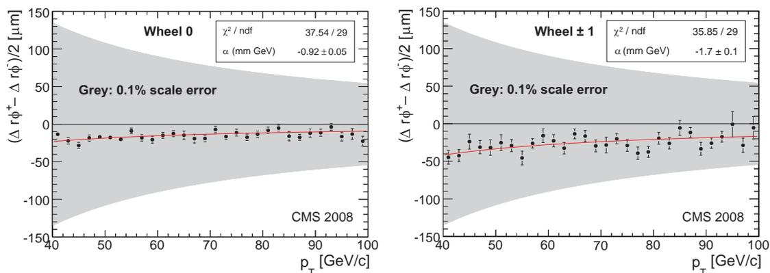
**Figure 2.** Residual distances, in the bending plane, between the extrapolation of the tracker tracks and the measurements in the first muon station, for the CRAFT cosmic muon data set, as a function of the transverse momentum. Left: wheel 0. Right: wheels  $\pm 1$ . The shaded area shows the expected effect of a 0.1% distortion of the field map in the region between the inner tracker and the coil. The solid line represents a fit to the function  $\alpha/p_T$ .
