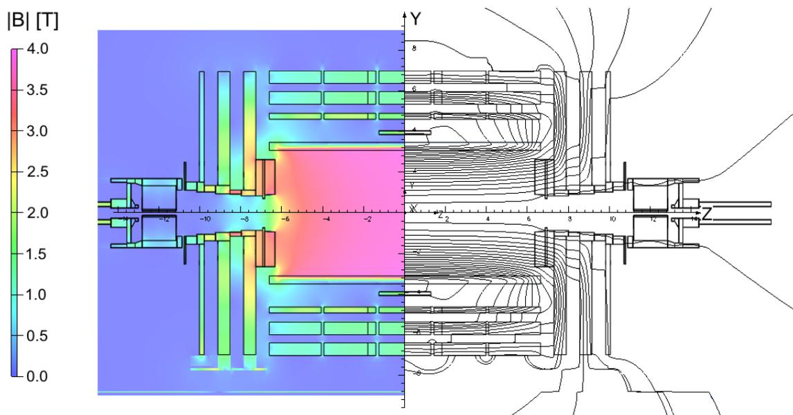
**Figure 5.** Value of  $|B|$  (left) and field lines (right) predicted on a longitudinal section of the CMS detector, for the underground model at a central magnetic flux density of 3.8 T. Each field line represents a magnetic flux increment of 6 Wb.
