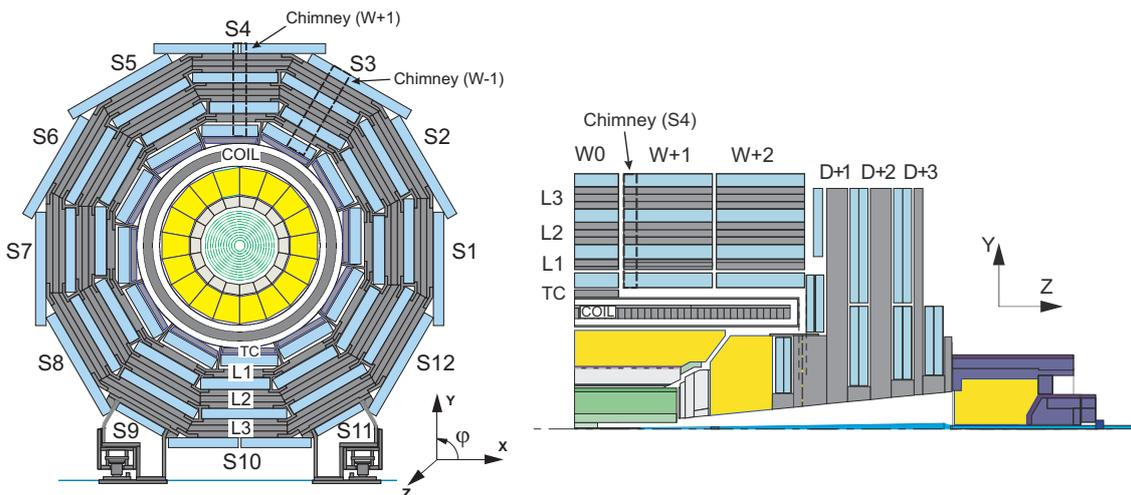
**Figure 1.** Schematic views of the CMS detector, with the numbering convention for azimuthal sectors (S), wheels (W), barrel yoke layers (L) and endcap disks (D). “TC” is the “tail catcher”, an additional steel layer present in the central barrel wheel only. Left: transverse view at  $z = 0$ . Right: longitudinal view of one quarter of the detector. Wheels on the  $z < 0$  side (not shown) are labeled W-1 and W-2. The location of the “chimneys” described in section 3 is indicated with boxes.
