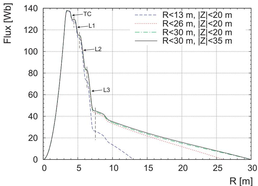
**Figure 6.** Magnetic flux through a disk of radius  $R$  in the transverse plane at  $z = 0$  m, as predicted by the TOSCA model for the surface configuration and 4 T operating conditions, computed within different enclosing regions. The vertical dashed lines indicate the location of the four barrel muon stations.
